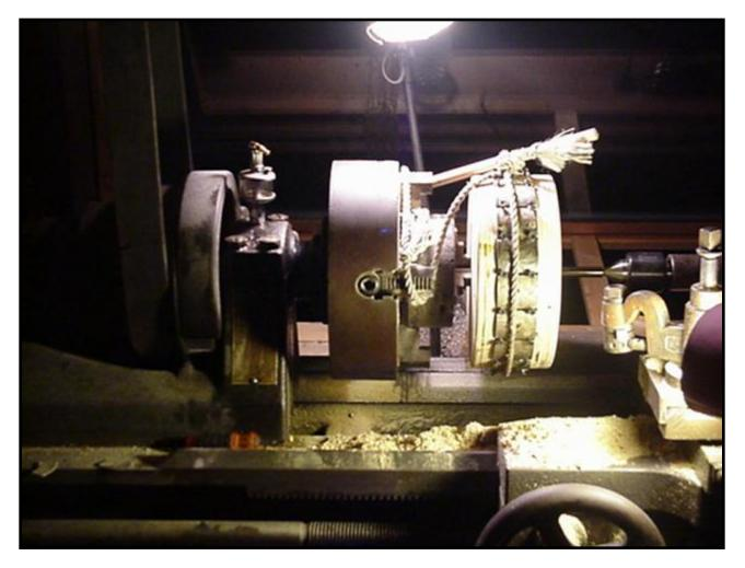
On the metal lathe (a wood lathe would work fine) I evened up the armature so that the diameter is approx 8.75". In the center of the armature I cut a slot 3/16" deep exactly wide enough to accept the magnets (1.74"). The magnets are laid in with alternating poles facing up. This particular magnet is available with either North or South on the outside. This alternator requires 9 of each variety. The diameter is such
