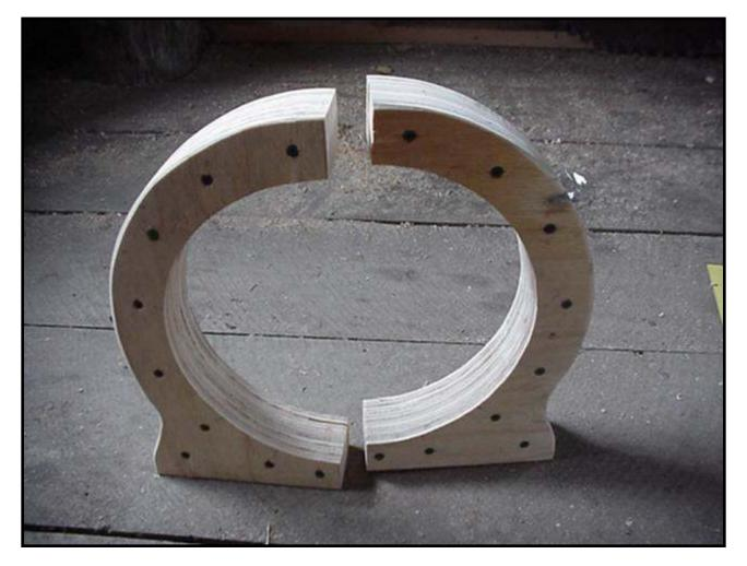
The stator (that part which will eventually hold the coils of wire) is built up of 3/4" plywood. The inner circle has radius of 5", which leaves room for coils between it, and the armature. The magnets protrude from the wooden alternator approx 1/8", so
