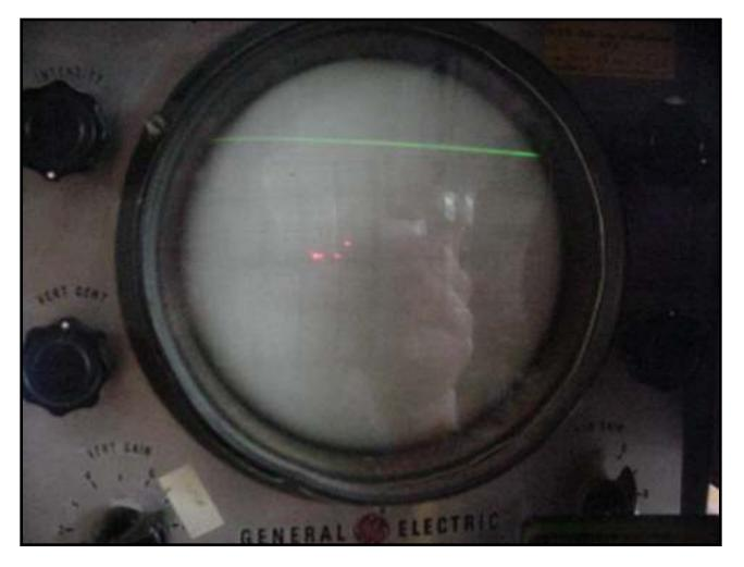
See above the nice, flat DC output after a capacitor is hooked up between Pos and Neg outputs.
