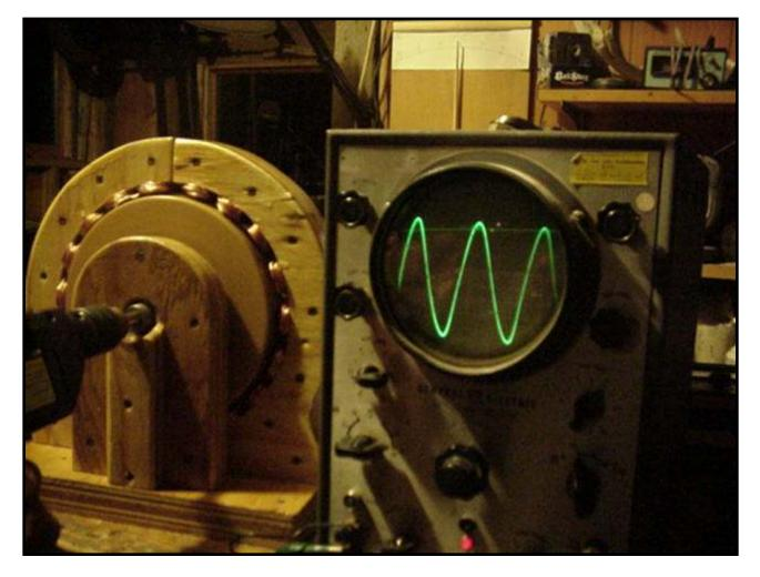
I was curious what the output would look like on the scope, considering the close proximity to one another of the magnets, and the "lumpy" armature. Keep in mind, what is shown above on the scope, is Alternating Current, directly out of the alternator. In order to be useful in batterycharging, it must be rectified into Direct Current. To do this a "bridge rectifier" (a simple arrangment of 6 diodes) must be used.
