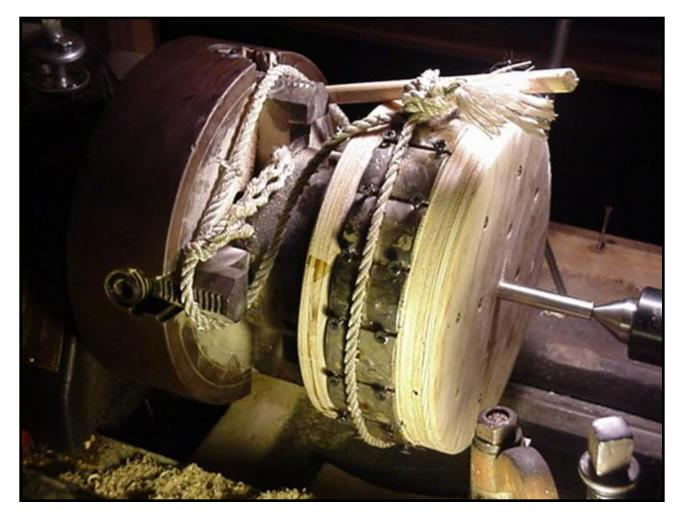
Once all the magnets were pressed in place, properly spaced with screws, I glued them in with epoxy. As a clamp, I simply tied a rope around the magnets and tightened it with a stick through the knot. When the glue started to set up hard, I removed the screws and applied a new coat of glue over the entire surface of the alternator. This not only aids in holding down the magnets, but it will protect the alternator from moisture.
