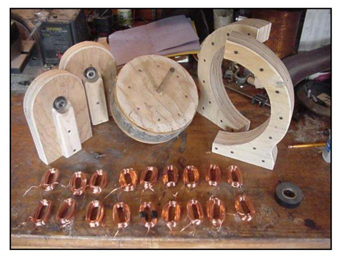
In the above image you can see all the parts of the alternator ready for finishing and assembly.
