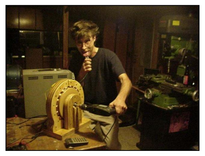
All the coils on each half of the stator are wired together in series. At that point, each half can be hooked in either series or parallel to most appropriately match the load with the alternator. Above is pictured the good old Taste Test, a sure fire way to test any battery, or generator, as long as it stays below about 10 volts! (otherwise it hurts--don't try this at home!)
