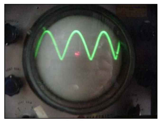
Shown above is the "rectified" output of the alternator. This is useful for battery charging, but - you'll notice how "lumpy" the Direct Current looks on the scope. Although this rarely causes problems, occasionally this sort of Direct Current will cause problems with radio and television reception (you'll hear a whine). To help smooth out the Direct Current available here, a capacitor can be used.
