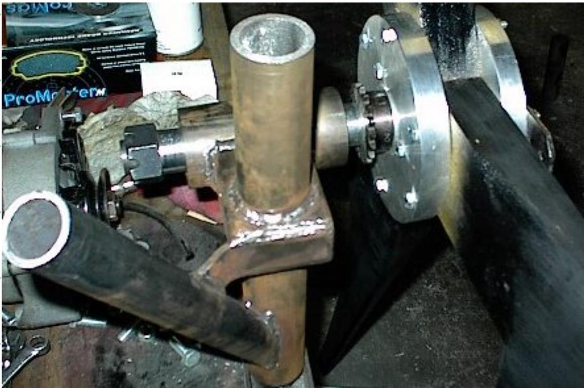
The only thing that was modified from his original version is the bearing head. Mine had to use the modified Gm alternator instead of the "brake drum"
