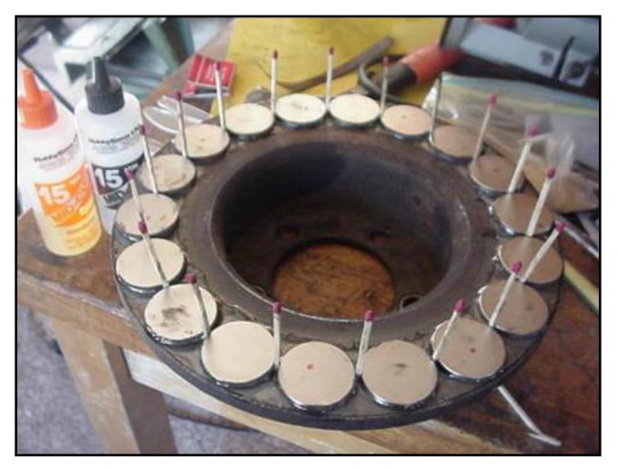
While I had the glue out, I glued the magnets into the brake disk at the same time. Once the glue set up partially, I removed the matchstick spacers.
