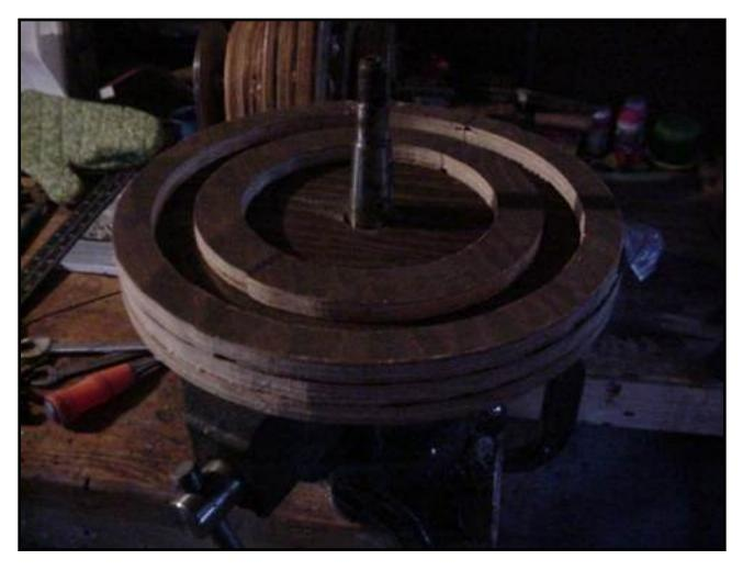
Pictured above is the beginning of the plywood stator. It is made out of laminated plywood discs. The total thickness is 1.5". The top layer, which is 1/2" thick, has a slot 1" wide at about 10" diameter so that steel laminates can be epoxied in. Over that will be the coils. (you'll see this later in the page!)
