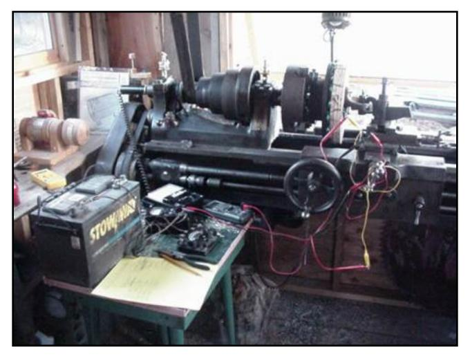
Pictured above is the "test rig." It's somewhat limited by the motor on my lathe - the max speed I could test it at was 500 rpm, and even at that speed it loads up the motor and slows it down. The problem is that my lathe only has a 1/2 hp motor on it. The reason for this is that I run my whole shop off my batteries and a "cheap Chinese" inverter! Someday I'll upgrade to a 1 hp motor, which my inverter should barely run...but for now my tests are limited.
