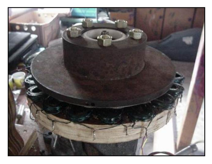
The completed unit. It's already been attached to a homebrew wind generator with an 8-foot diameter, 3-bladed rotor--and is up and flying! <u>See it HERE!</u> We've already seen peaks of over 60 amps into a 12 volt battery bank, and it survived 60-mph winds last week. Steady output of 30 amps in 28 mph winds, and reaches charging voltage at around 12 mph.
