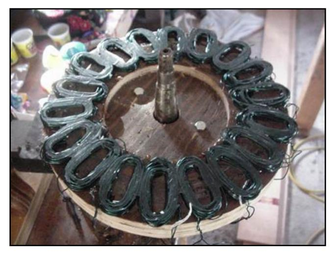
Above is pictured the stator, mostly complete, with the coils smashed down tightly and glued well. At this point, I coated the assembly (plywood front and back) with epoxy to weather proof it as best I could. I divided the coils in half, hooking 2 sets of 9 coils together in series and figured I would decide later whether to hook the two halves in series or parallel - this was not decided untill a prop was made and I actually got to test it in known windspeeds.
