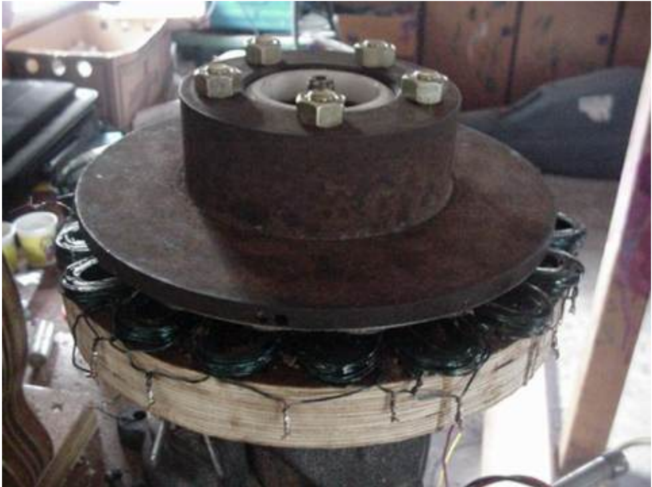
Homemade Volvo Brake Disc PM alternator, 800 watts, $150!
