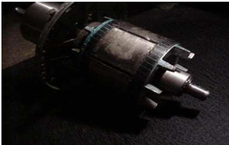
Armature converted with permanent magnets
