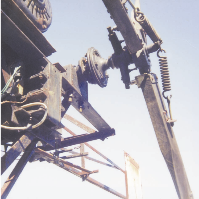
Detail of the underside of the drive shaft mounting. The furling tail is visible in the background.
