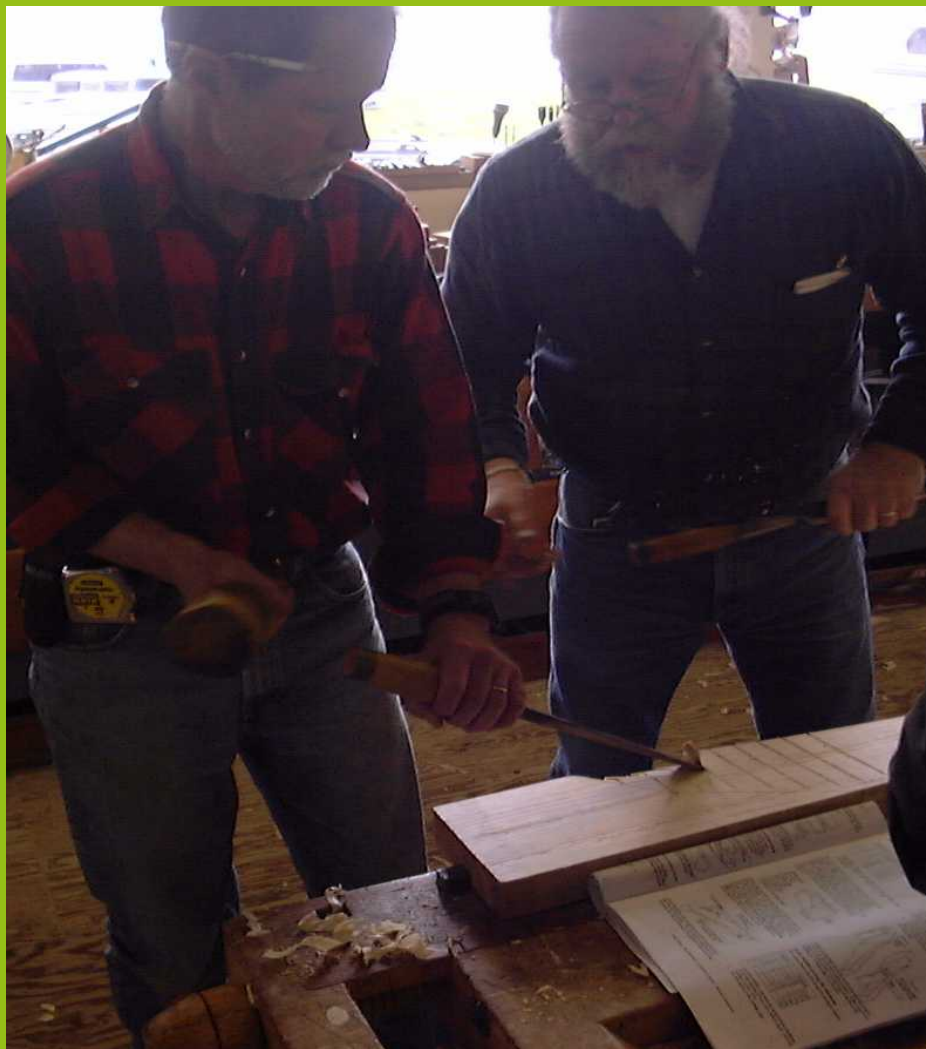
The slow approach is to kerf the wood out by cross-cutting.
