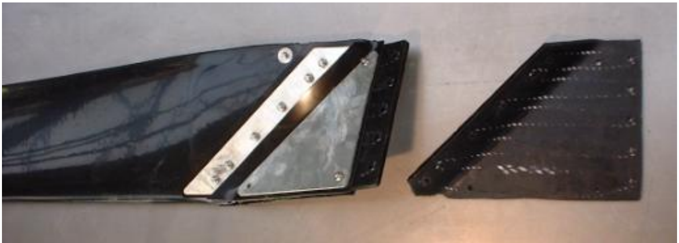
Figure 2: PU Hinge separate and integrated into the blade root.
