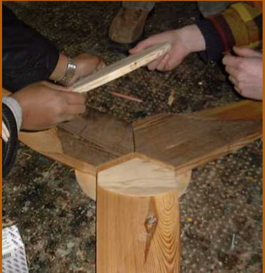
Fitting the back disk to the blades
