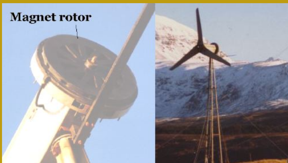
In this picture you can see the magnet rotor inside the alternator. The cover was removed to improve cooling, and it looks nice too, wheeling along.
