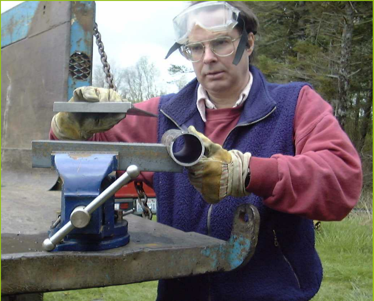
Brett making the alternator mounting brackets. Note the large hole for the bearing housing (below).
