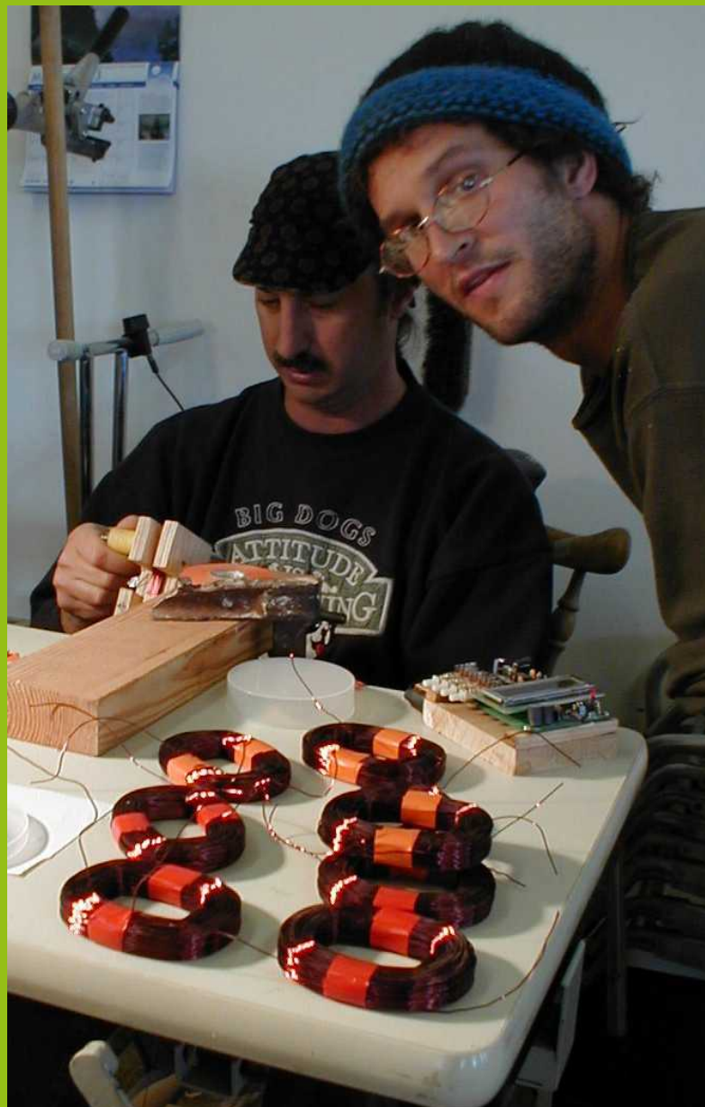
Coil winding. Andy Swingler at work. Aaron and Dylan piling up coils.
