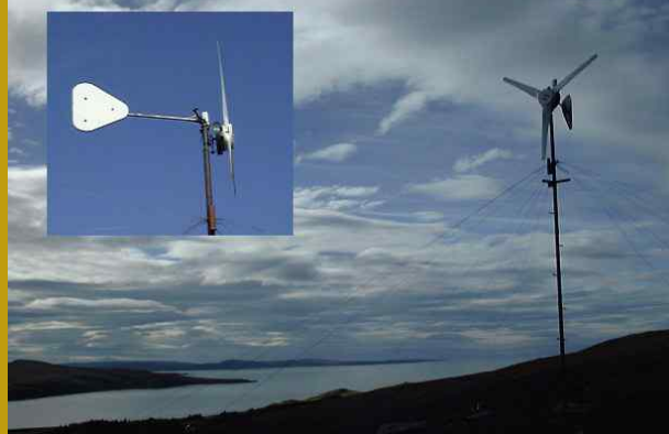
ITDG alternator on test at Scoraig September 1999
