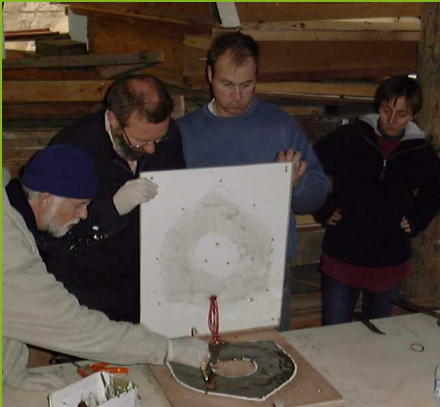
Painting the magnet disks with resin
