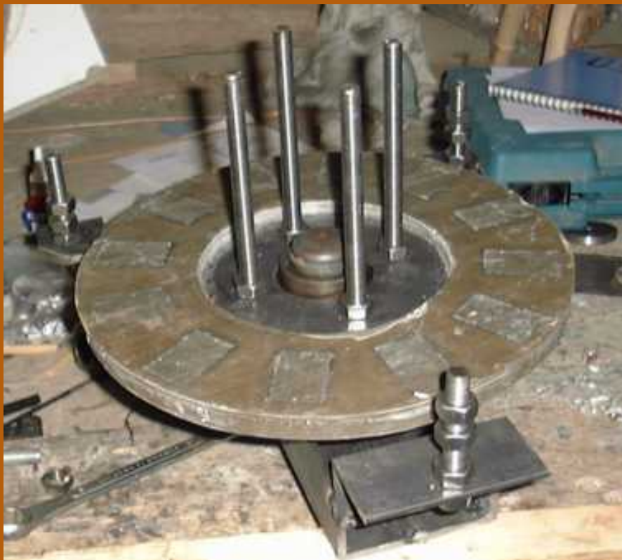
Using the jacking screws to lower the front rotor into place gently
