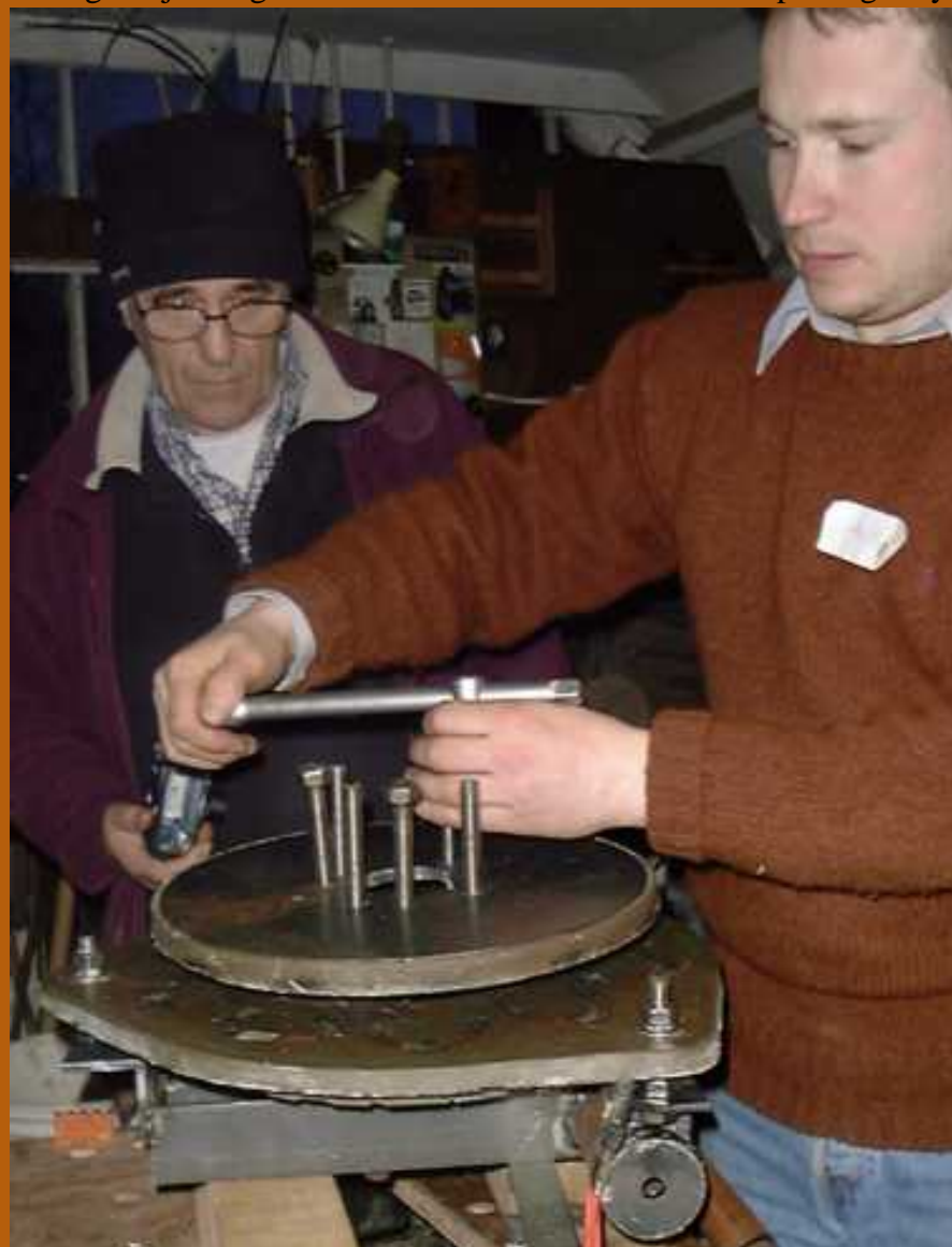
Using the jacking screws to lower the front rotor into place gently
