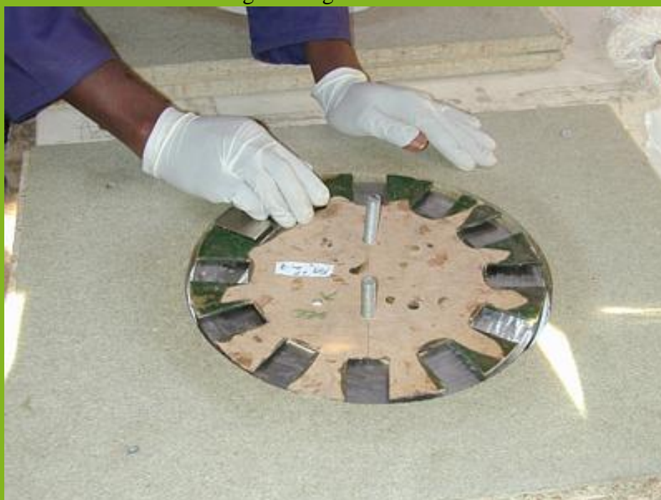
Fitting the magnets on the disk
