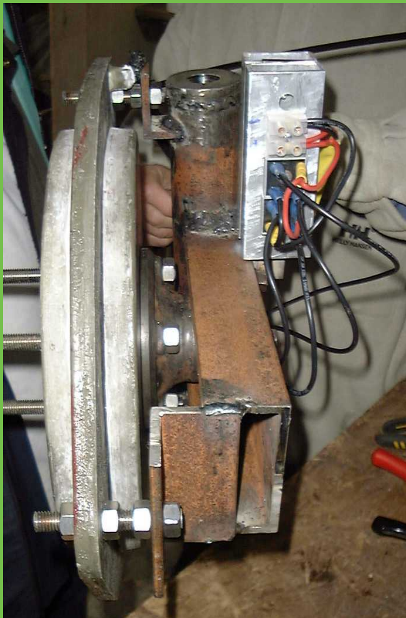
Pic 25: While Julius Tangka is trying to "rip off" the insulation, John and Stephan are checking the tail movement. We had to weld a small additional piece of steel to prevent the tail from hitting the hinge pipe weld.
