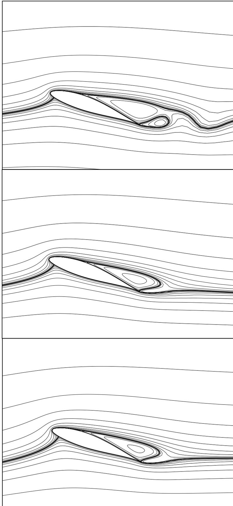
Figure 4-3 Stream lines for the flow around a NACA 63<sub>2</sub>-415 airfoil at incidence 20° and  $Re=1.5 \times 10^6$ , (a) 2D, (b)  $k=6$ , (c)  $k=4$ .
