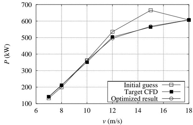
Figure 3-6 Mechanical power for optimised result compared with initial guess and target CFD.
