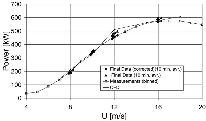
Figure 2-23 Calculated 10-minute average power based on 'Final Data' and 'Final Data (corrected)'. They are compared to power curves from measurements and CFD.
