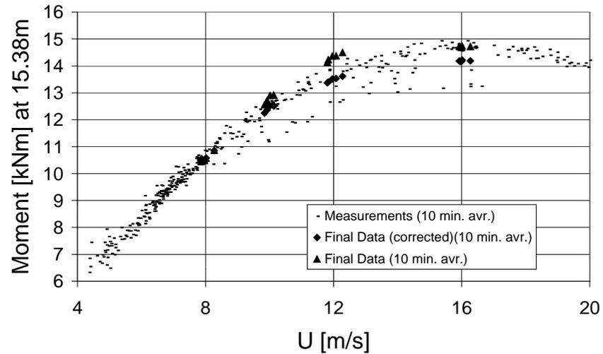
Figure 2-26 Computed flap moments in  $r=15.38$  m,  $0.75R$ , using 'Final Data' and 'Final Data (corrected)'. Comparison with measured flap moments.
