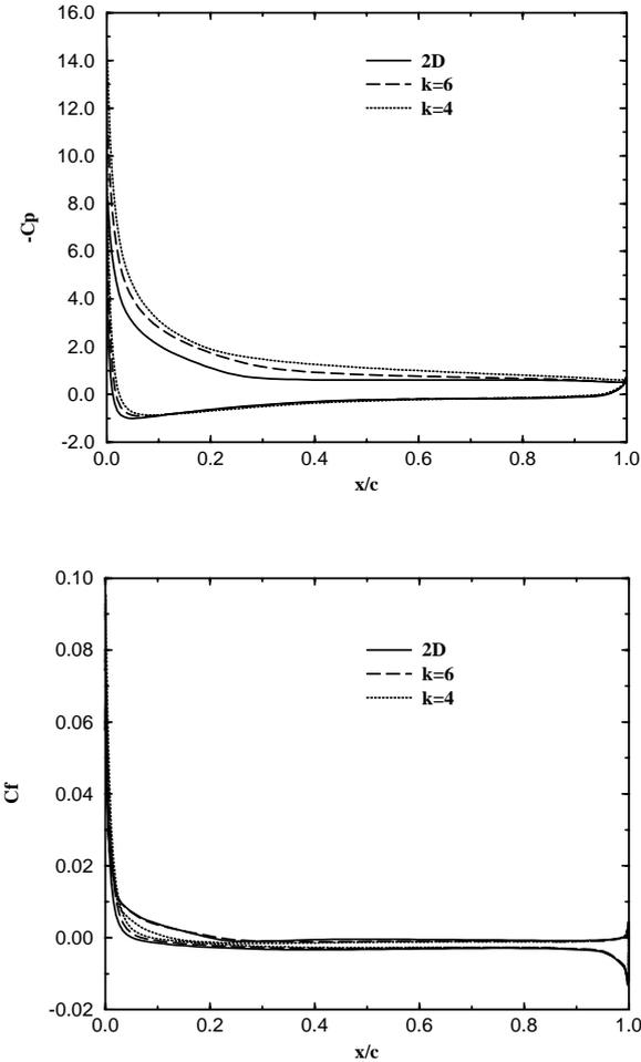
Figure 4-4  $C_p$  and  $C_f$  distributions on a NACA 63<sub>2</sub>-415 airfoil at incidence  $20^\circ$  and  $Re=1.5 \times 10^6$ .
