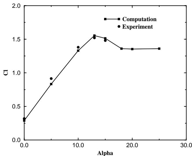
Figure 4-2 Comparison of computed 2D  $C_L$ -coefficient vs.  $\alpha$  of a NACA 63<sub>2</sub>-415 airfoil at  $Re = 1.5 \times 10^6$  with experimental data at  $Re = 3 \times 10^6$ .
