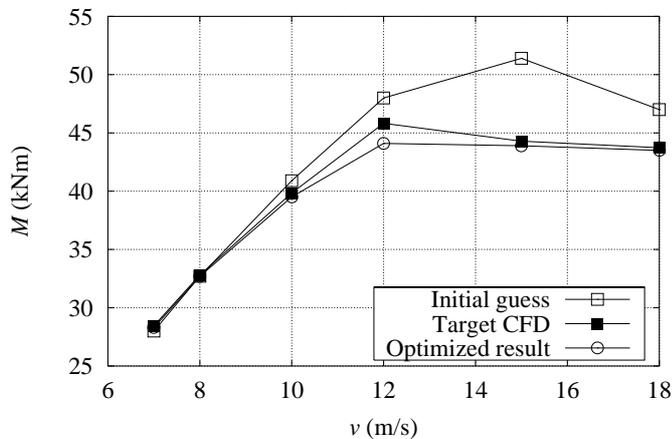
Figure 3-9 Blade bending moment around the chord axis at  $r = 12.5$  m for optimised result compared with initial guess and target CFD.
