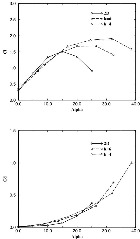
Figure 4-5  $C_L$  and  $C_D$  vs.  $\alpha$  of a NACA 63<sub>2</sub>-415 airfoil at  $Re=1.5 \times 10^6$ .
