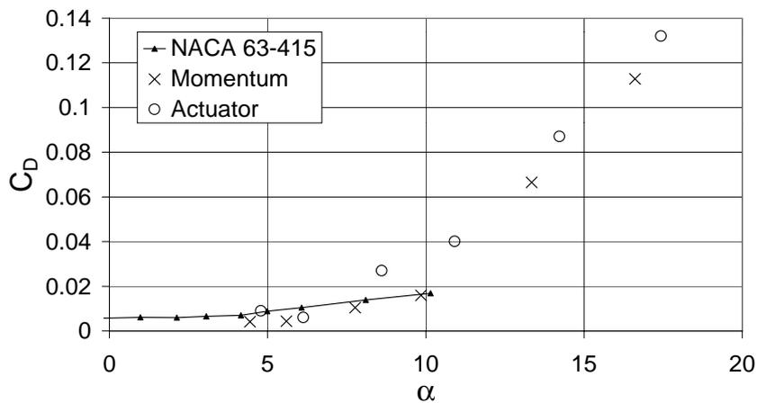
Figure 2-12 Derived  $C_D$  at  $r=19.0$  m ( $t/c=15.75\%$ ) using momentum theory and actuator disc theory. Comparison with 2D wind tunnel measurements.
