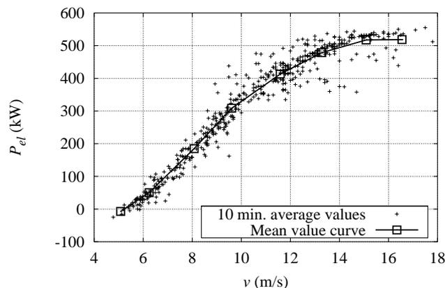
Figure 3-10 Measured electric power 10-minute average values and average value curve.
