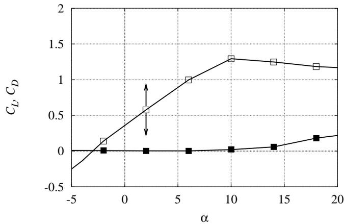
Figure 3-1 Parametric curves that describe  $C_L$  and  $C_D$  versus  $\alpha$ . The discrete points are design variables.
