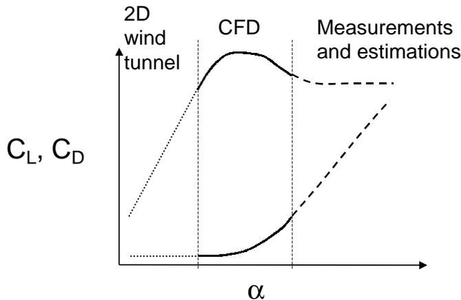
Figure 2-6 Sketch of the construction of airfoil characteristics.
