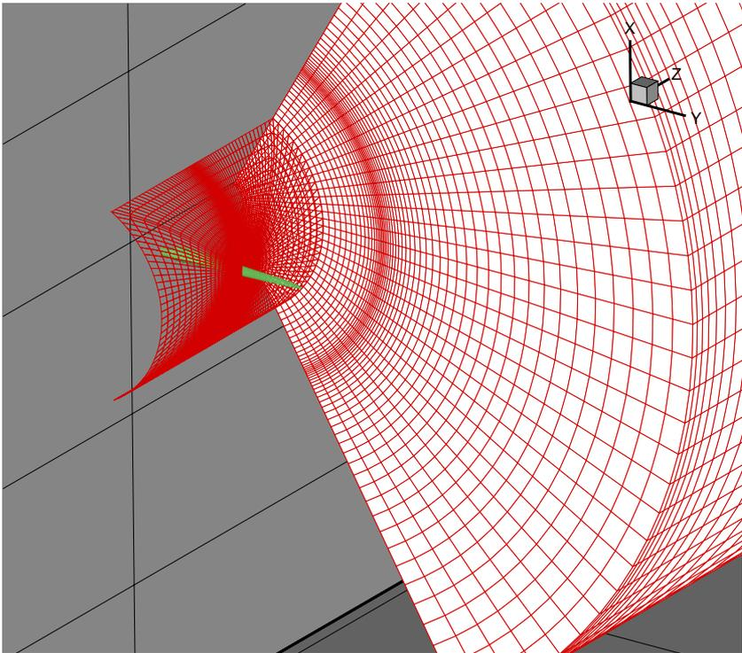
Figure 2-1 Mesh of the 120 degrees section of the three-bladed rotor. The blade is seen to the left and the outer boundary is seen to the right.
