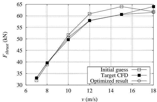
Figure 3-7 Rotor thrust force for optimised result compared with initial guess and target CFD.
