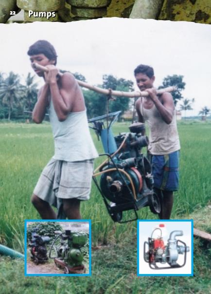
"Improved motor pumps of 2.5 HP yield as much water as traditional 5 HP pumps, for half the fuel consumption".
