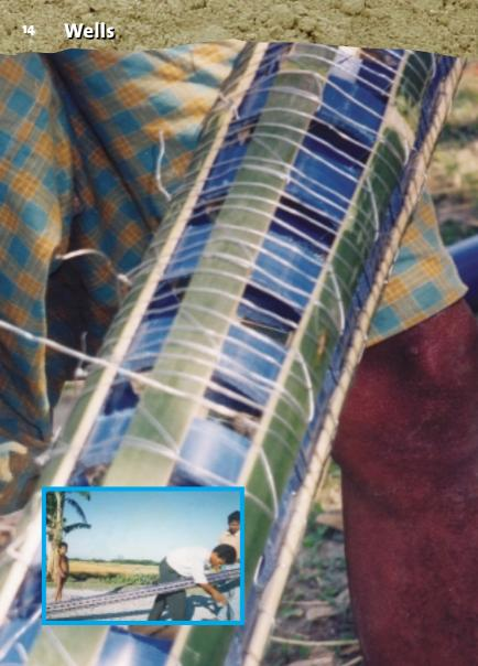
"The fuel consumption of irrigation pumps was decreased by 40% through the use of improved bamboo screens".
