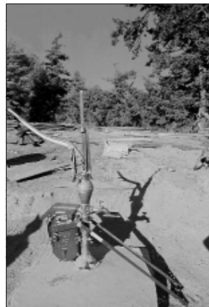
ram is a water-powered device. (Fig. 10) It has one function: to pump water.
