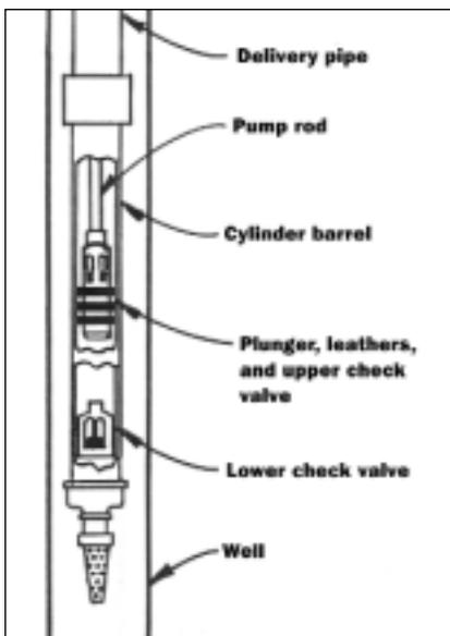
Figure 5: A deep well piston pump and cylinder.
