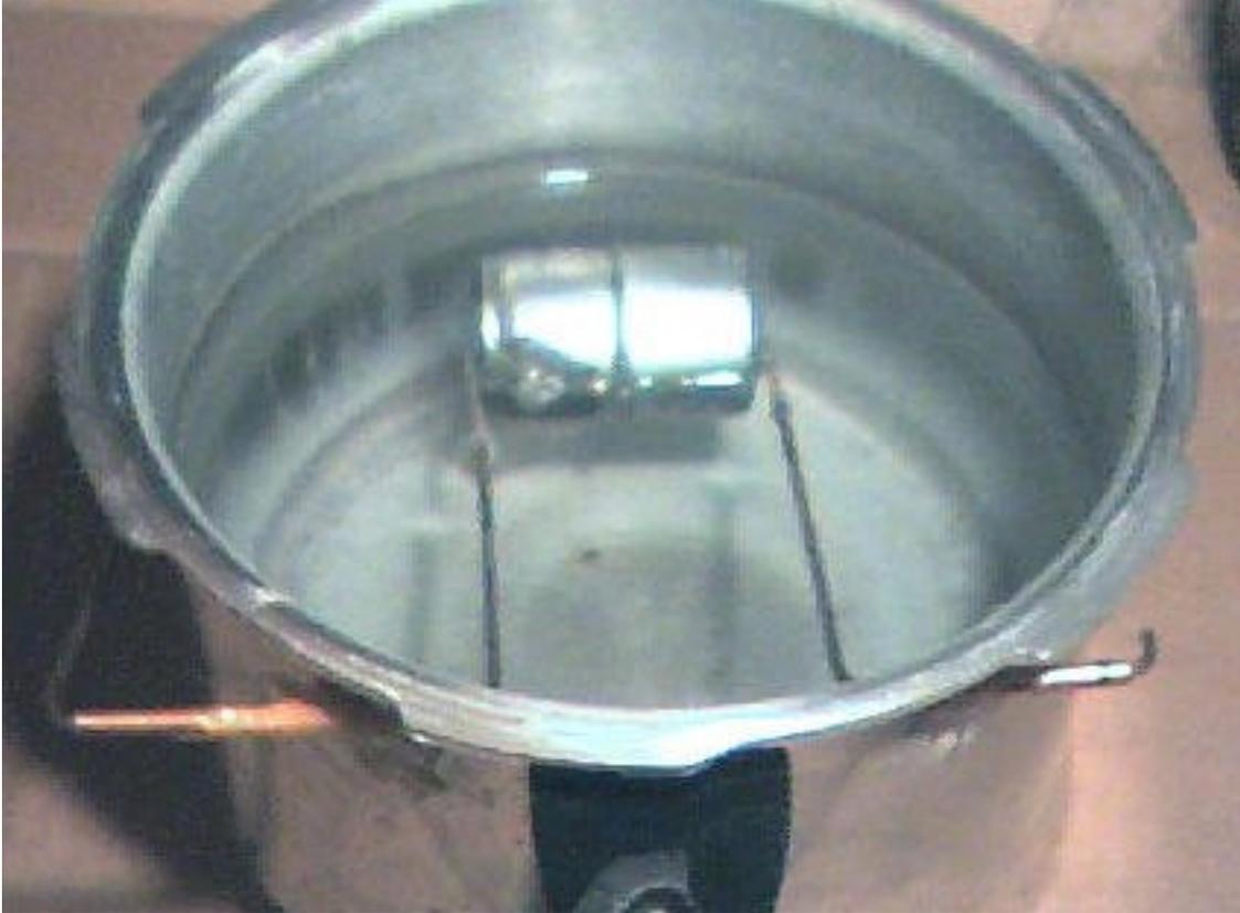
3/32" Brass brazing rod was used for the float hinge mechanism. Any other type of wire would also have worked including coat hanger wire. Small copper pipe about 3/16 inch was used for the outer hinge and was epoxied to the aluminum pot by use of copper epoxy. The copper epoxy is designed to replace solder and is sold at home improvement stores like Home Depot.
