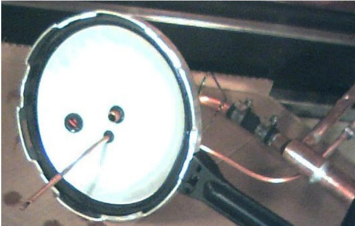
A rubber grommet from the firewall or from the PVC valve from a junk after PS car may be able to be used. The grommet used for the safety valve in the pressure cooker may be able to be used. By the way I found the new “step drill bits” to be quite usefully in drilling the hole in the lid of the pressure cooker and when needed in the side near the bottom for supply 5 gallon buckets.
