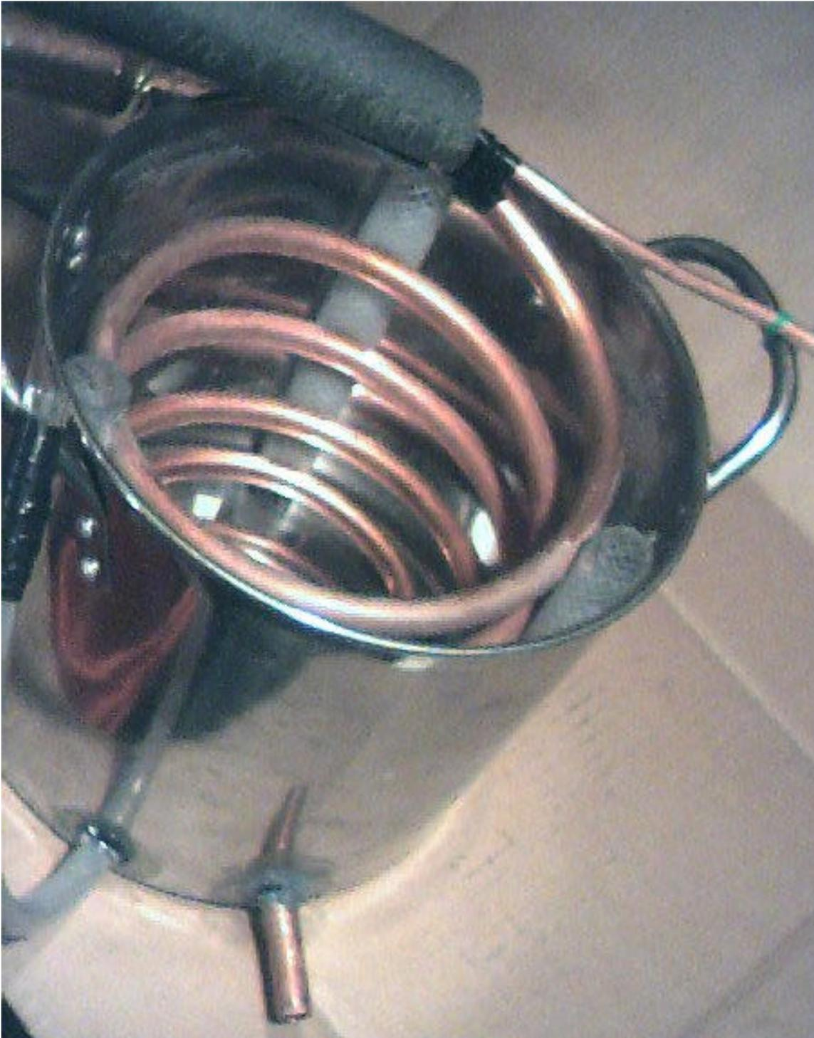
I was able to produce about 6.5 cups/hour of distilled water. The input source was an electric stove 240 volt x 7.3 amps = 1750 watts. Note that water is replenished from the upper reservoir at the same rate it is turned to steam by adjusting the needle valve on the
