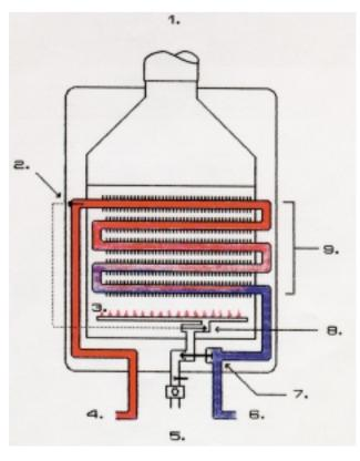
(1) Gas vent [flue]. (2) Thermostat sensor. (3) Burner.
