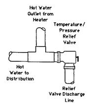
To install a temperature/pressure relief valve on a tankless hot water heater, use a T fitting in the hot water outlet line as shown.
