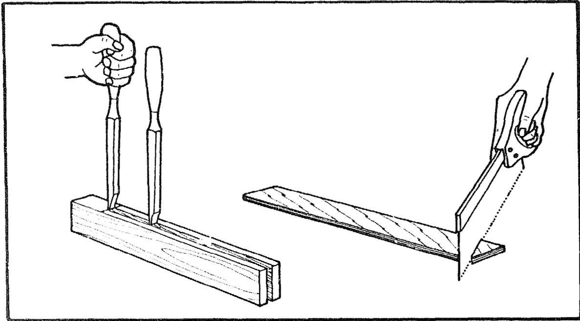
Use a 6mm chisel to cut out the waste wood in the stock.
