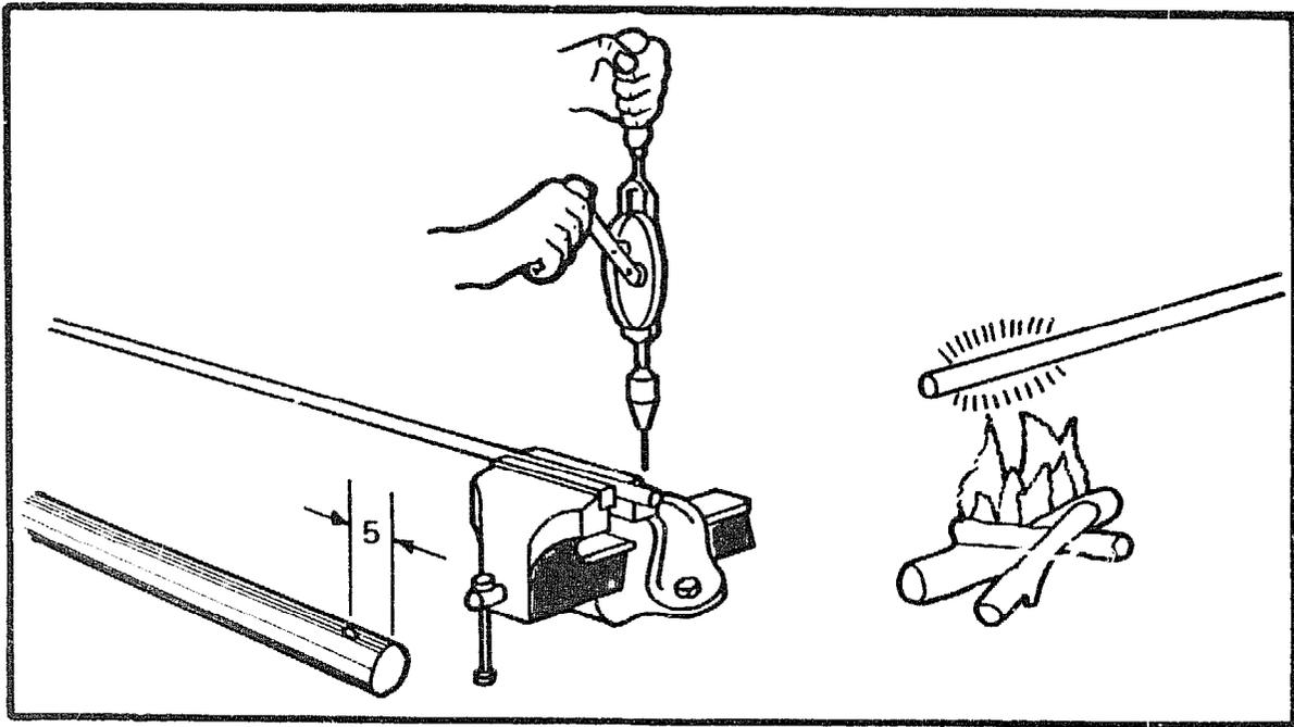
Centre punch and drill a  $\text{Ø}3\text{mm}$  hole in one end of the steel rod (the hole should be slightly bigger than the nails to be used as blade holders). Build a fire from wood or charcoal. The frame can be bent easily if the rod is red hot.
