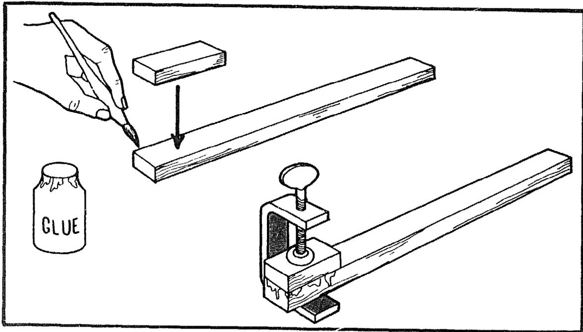
Take the pieces prepared to  $200\text{mm} \times 10\text{mm} \times 20\text{mm}$  and  $30\text{mm} \times 10\text{mm} \times 20\text{mm}$ . Glue and clamp the smaller one to the end of the larger one, and make sure there are no overhangs. Plane the glue off when it is dry.
