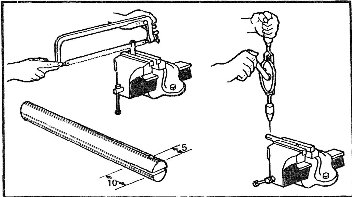
Take the two pieces of 9mm bar and saw a slot 10mm long in one end. 5mm in from the same end, punch and drill a  $\varnothing 3\text{mm}$  hole right through.
