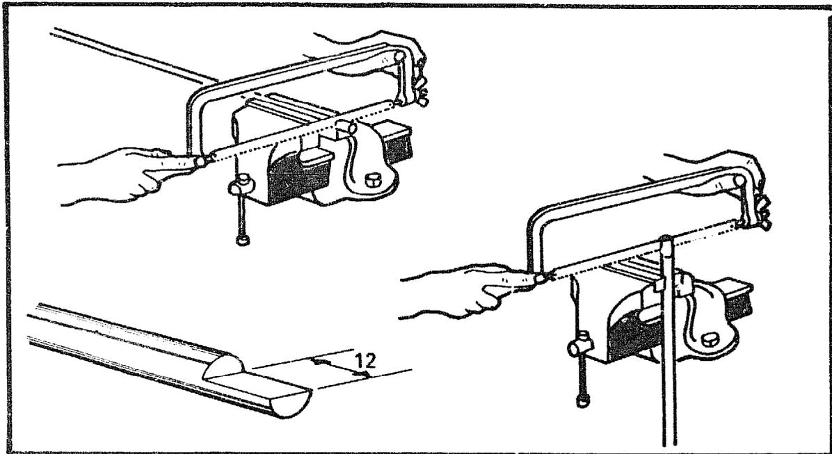
Take the rod and saw out a semi-circular section 12mm long, using a hack saw.
