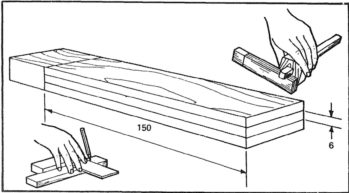
Take the timber prepared for the stock and square a line round 150mm from one end.
