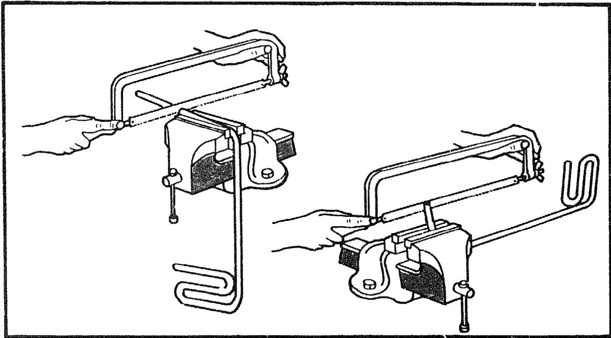
Measure and cut the front leg of the frame to the same length as the leg at the handle. Saw a slot down the middle of the front leg 12mm long with a hack saw.
