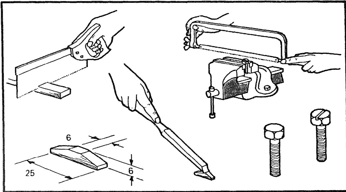
Take the timber prepared to make the wedge and the shoe and cut a small piece off 25mm × 6mm × 6mm. Shape the shoe as shown with a chisel. Take the 20mm × 6mm bolt and saw a slot in the head for a screwdriver.
