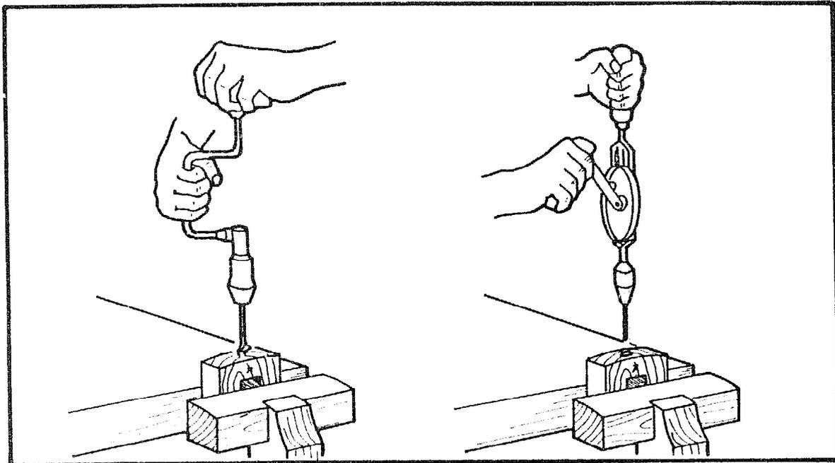
With a 12mm drill bit bore a hole on the centre mark to a depth of 6mm. Now drill a  $\varnothing 6\text{mm}$  hole right through, into the recess cut for the shoe.
