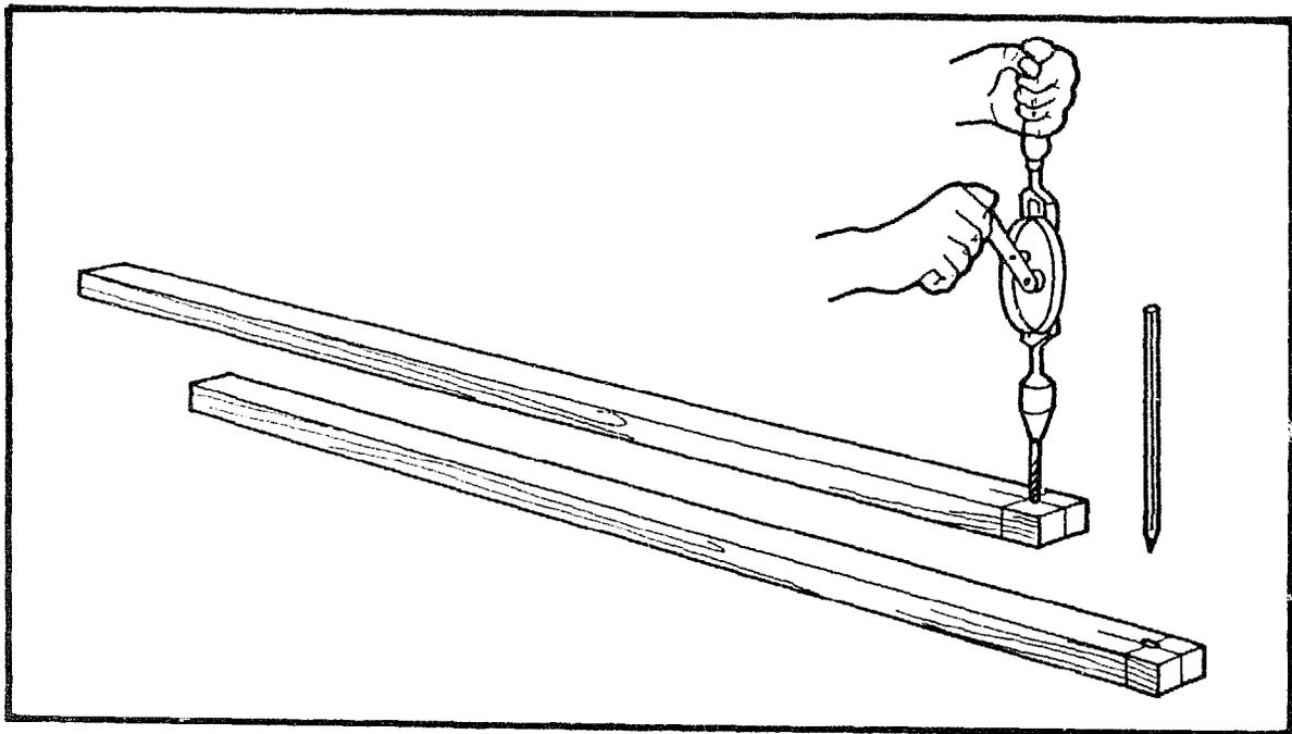
Drill a  $\varnothing 8\text{mm}$  hole from both sides of the stem. Fit a pencil into the hole
