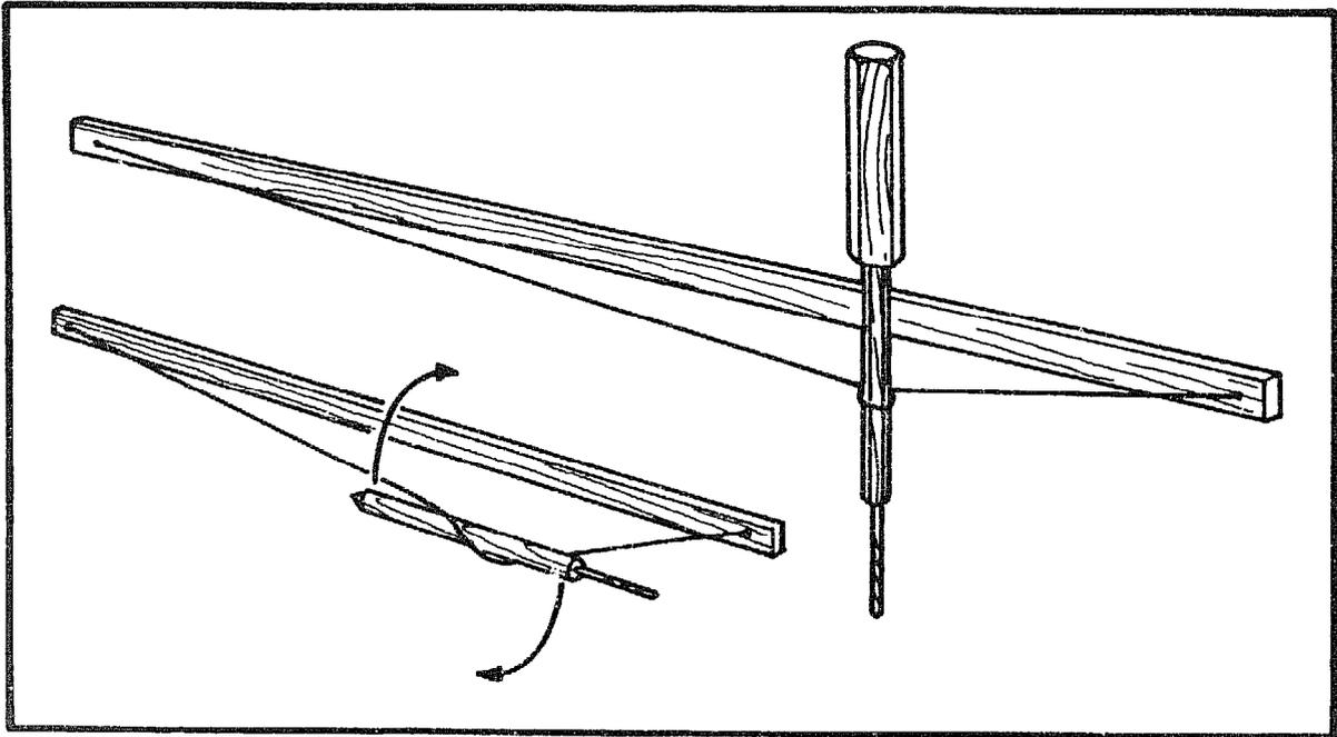
Twist the bow string once around the stock of the drill. Put some grease or cooking fat on the point, and push it into the hole in the handle.
