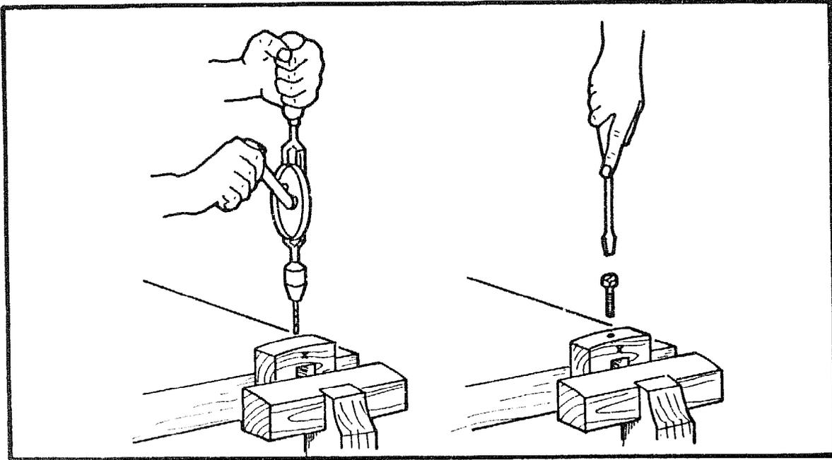
Mark the centre of the top of the fence, and drill a  $\varnothing 5\text{mm}$  pilot hole right through into the recess for the shoe. The pilot hole must not be drilled through the end grain.
