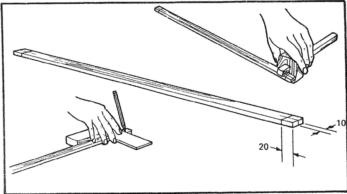
Take the timber prepared for the bow and square a line 20mm from both ends. Gauge a line in the centre of both ends to mark the holes for the bow string.
