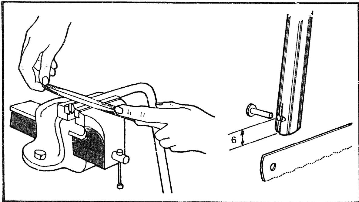
File a small nick, 6mm from the end of each leg, on the outside of the frame. This helps secure the blade holder. The blade holder is made from two cut-down 50mm nails.
