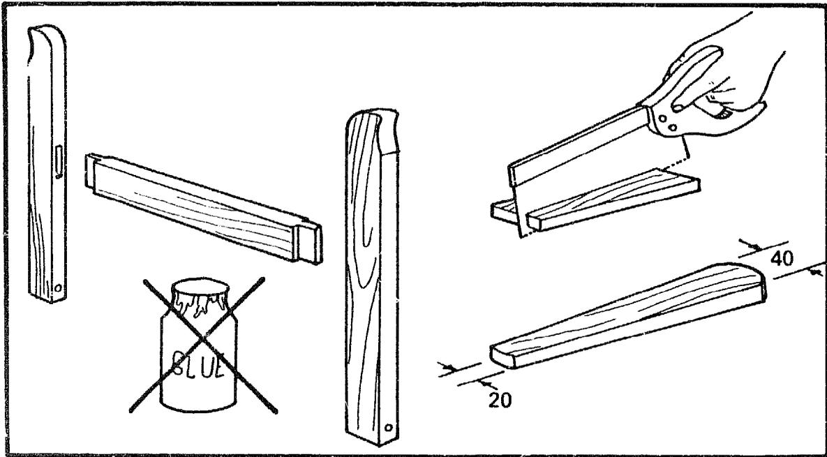
The joints should be a good tight fit, but they **MUST NOT BE GLUED**. Now cut and shape the twisting slat to the dimensions shown.
