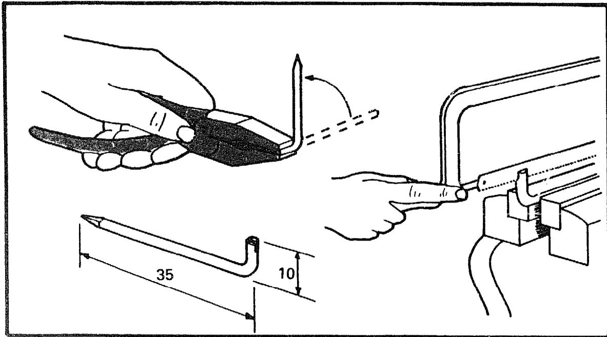
Saw the head off a 50mm nail leaving it 45mm long. Make a 90 degree bend 10mm from the sawn end. With a hack-saw carefully cut a slot about 4mm long down the centre of the nail.
