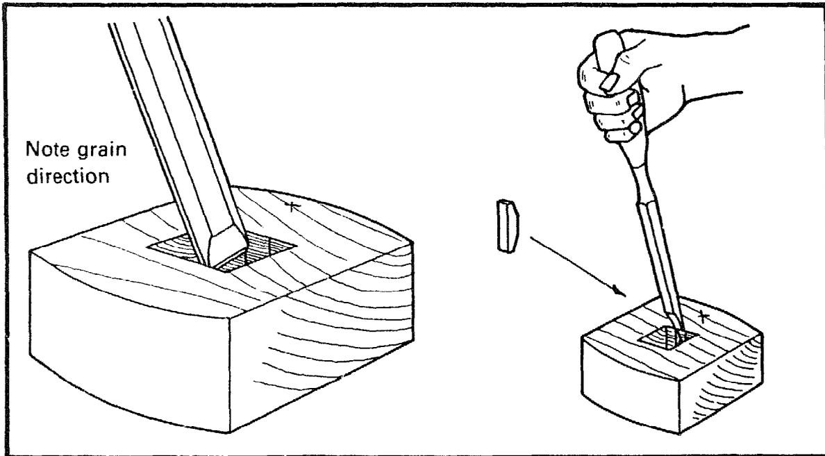
Make the fence as shown on pages 22 and 23, but do not cut the groove for the wedge. Instead carefully cut a recess in the centre of the mortise by first cutting the end grain with a chisel held at an angle. Then, with a 6mm chisel remove the waste.
