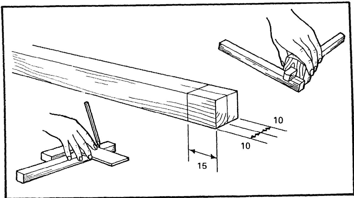
Take the timber prepared for the stem and square a line all round 15mm from the end. On two opposite sides of the stem gauge centre lines, crossing the pencil lines.
