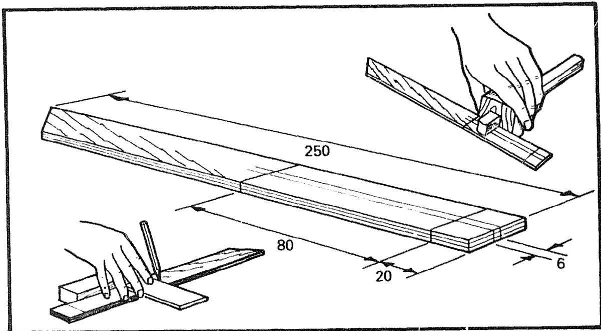
Prepare a piece of 6mm plywood 250mm × 40mm. Square a line 20mm from one end and another 100mm from the same end. Gauge a 6mm slot in the middle of the plywood between the two lines. Cut a 45 degree angle off the other end.
