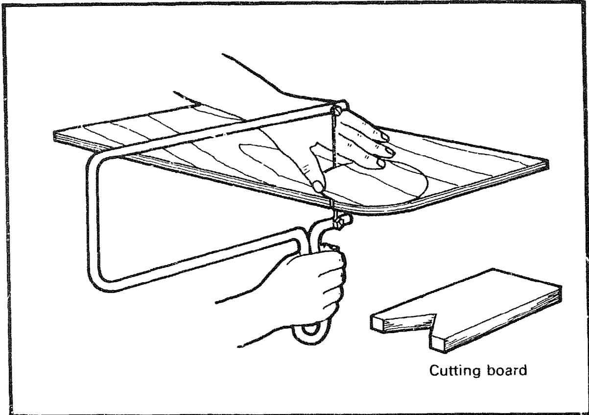
The fret saw is quite a specialized tool, not often used in carpentry workshops, but it is ideal for making childrens' toys and jig saw puzzles. The blade is very fine and is able to cut intricate shapes in thin timber and plywood, but it may be difficult to obtain. Unlike the coping saw, the blade cannot be adjusted, but this is overcome by the depth of the frame.
