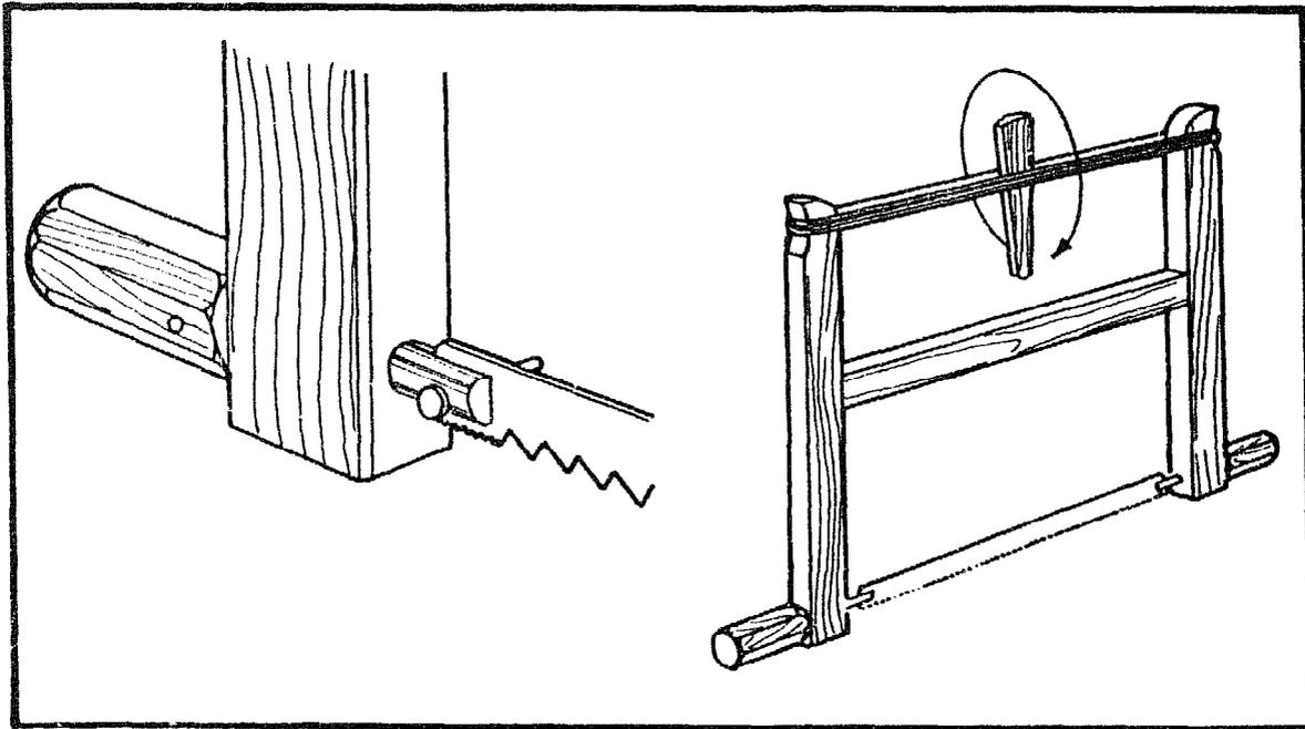
Now assemble the three parts of the frame. Push the blade sockets through the holes in the side frames and attach the blades with two 50mm nails cut down to about 20mm long. Wind some string three or four times around the top of the frame and tie the ends together. Slip the twisting slat through the string and twist it until the blade is tight, then slide it down until it rests on the crossbar.
