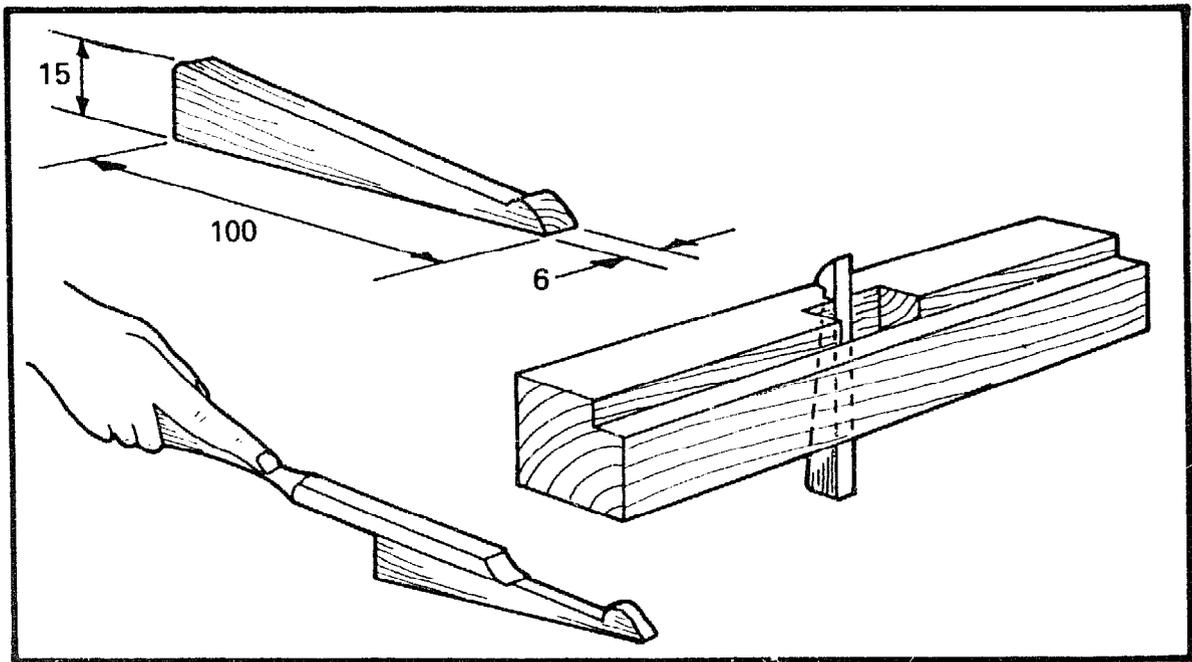
Cut the wedge to the dimensions shown, with a small knob at the end. This will stop the wedge falling out. Shape it so that it fits properly into the groove in the fence.
