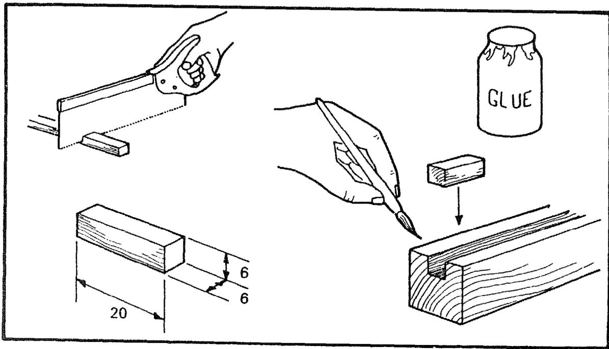
Cut a small block of wood from the piece prepared for the slider, 20mm × 6mm × 6mm. Fit and glue it into the groove at the end of the stem.
