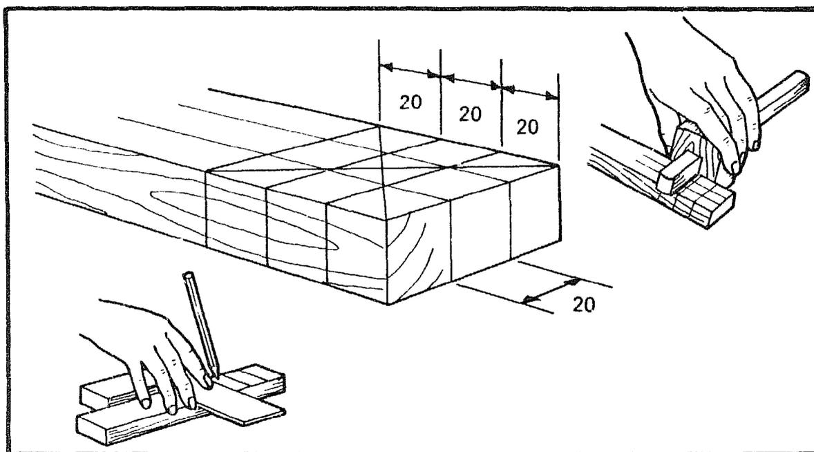
Take the timber prepared for the fence and square three pencil lines 20mm apart all round the timber; the first line should be 20mm from the end. Use a mortise gauge to mark two lines 20mm apart in the centre of the fence. Now mark the diagonals to find the centre of the mortise on both sides.
