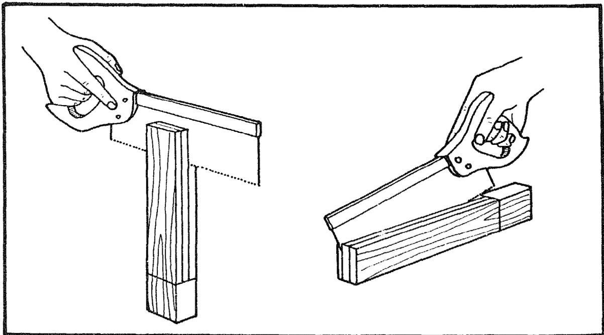
Use a tenon saw to saw out as much of the socket as possible.
