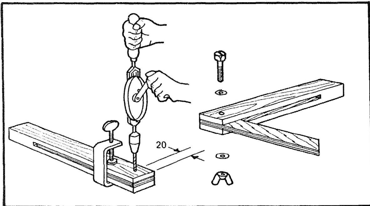
Fit the straight edge into the socket so there are no overlaps. Mark a central point 20mm from the end of the stock and drill a 6mm hole right through both pieces of wood.
