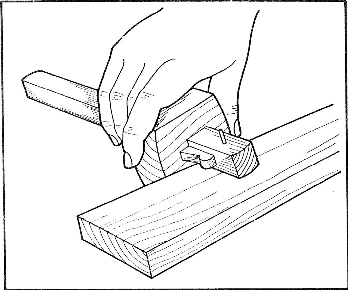
Marking gauges consist of two main parts, a fence and a stem. The stem carries a pointed metal spur at one end. The fence can be fixed to any position along the stem by a wedge as described here, or by a locking screw as shown on page 27 and page 41.
