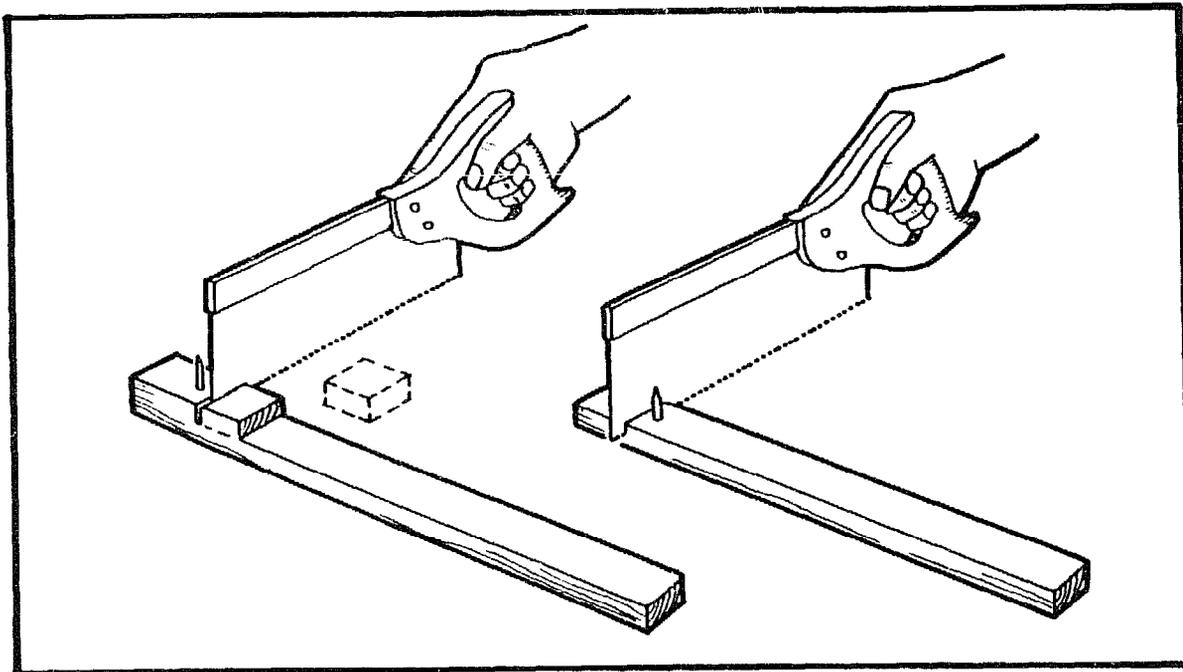
With a tenon saw, cut the step of stem **A** back to within 3mm of the spur. Also cut the end off stem **C** 3mm from the spur.
