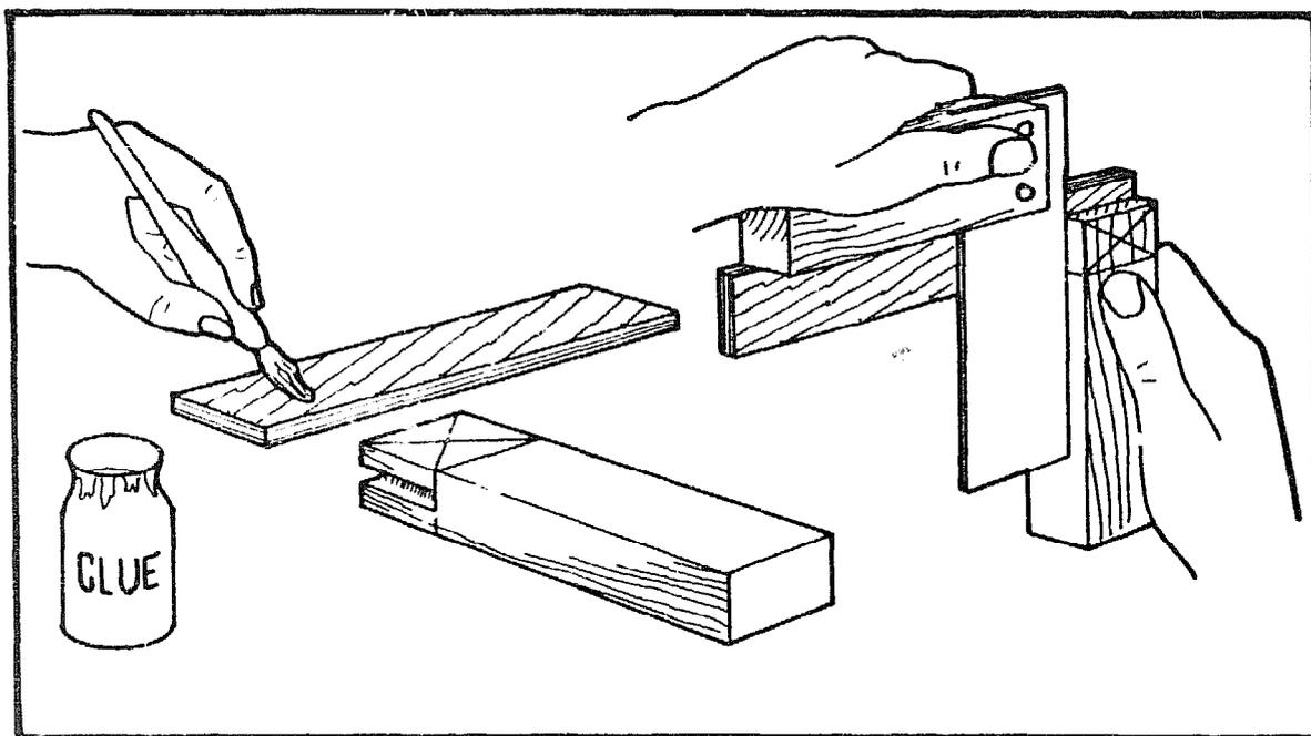
Glue the blade into the stock and, before the glue dries, make sure the blade and stock are square. Leave the assembly to dry.
