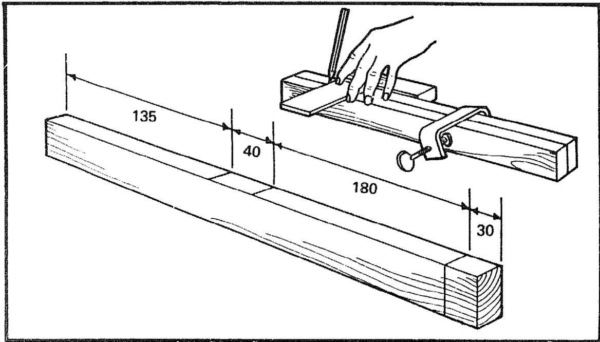
Clamp the two side frames together and square two lines across, 40mm apart, for the mortise. Square one line across, 30mm from the bottom, to mark the hole for the blade socket. Square this line all round both frames.
