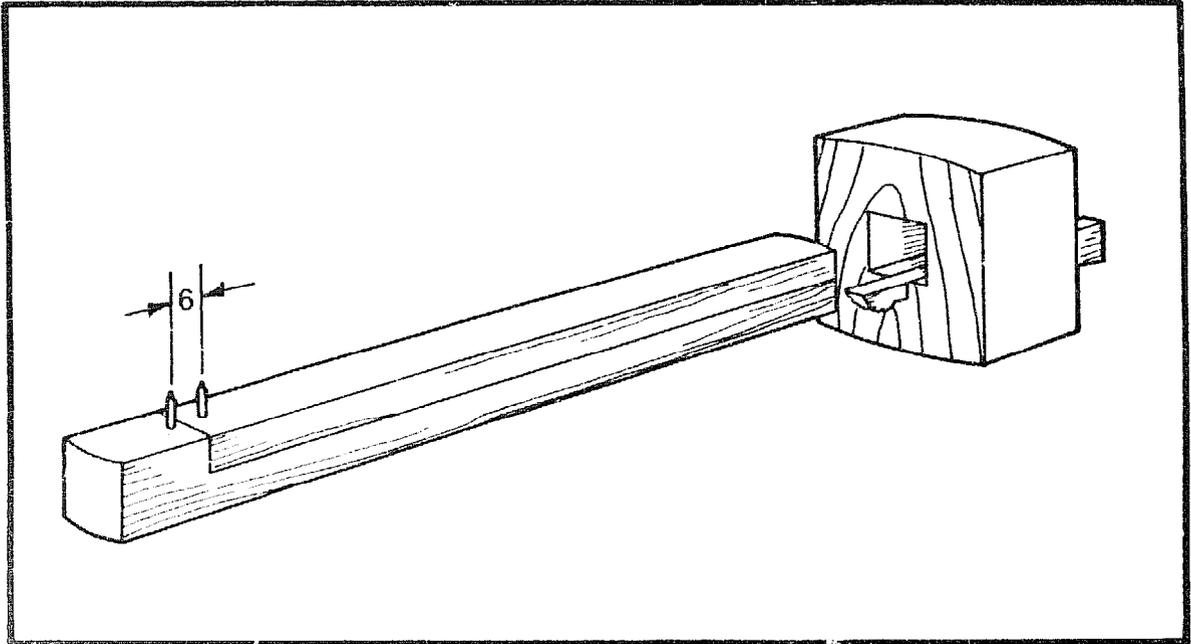
Fit the two parts of the stem together and if necessary trim the ends with a chisel or sharp knife so that the distance between the spurs is 6mm. Mark and cut the back end of stem **C** so that it is flush with the end of stem **A** and assemble the gauge.
