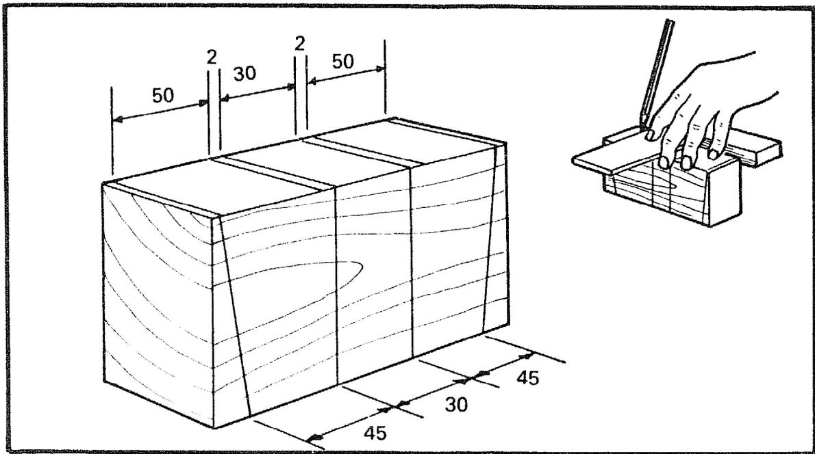
Square two lines 30mm apart in the centre of the block. On the top mark two lines 2mm towards the end. Now mark the angled ends of the mallet head, by squaring two lines 50mm towards each end, on the top, and two lines 45mm towards the end, on the bottom.
