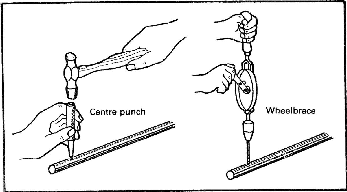
*Drilling a hole.* It is important to punch a small dent in the workpiece first. This will keep the drill bit from wandering off the mark.
