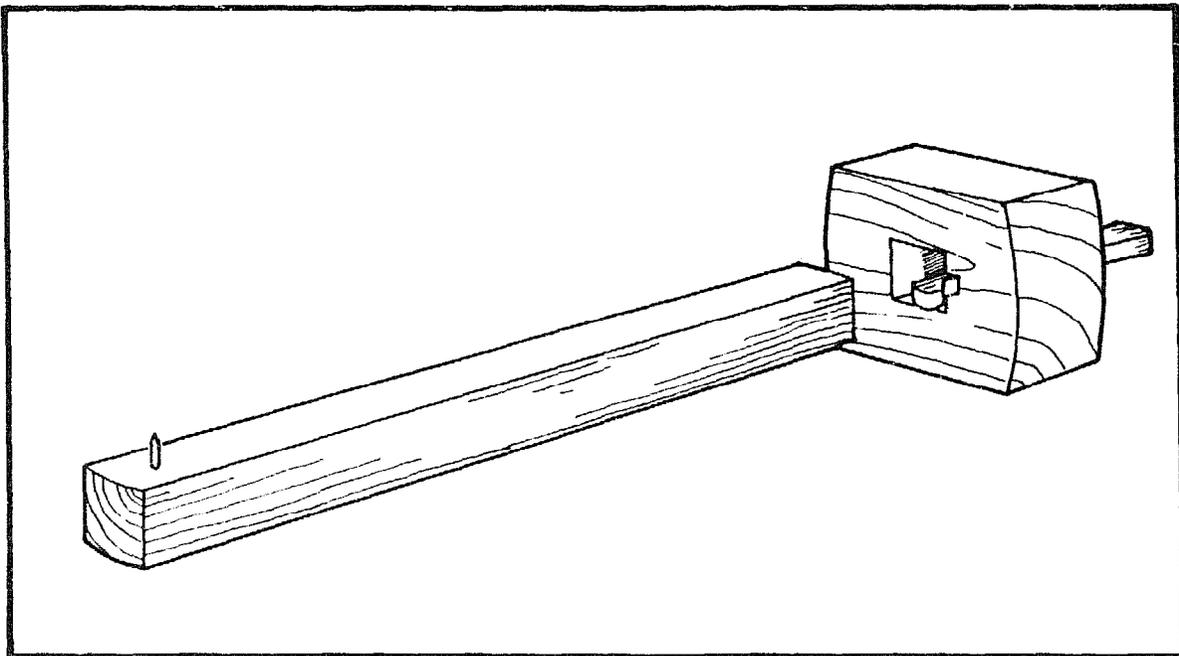
Assemble the marking gauge by fitting the wedge into its groove and sliding the stem through the fence. If it does not fit check that the sides of the mortise are straight, or plane the stem down very carefully.
