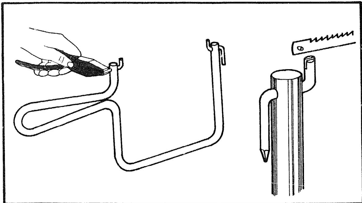
Push the sharp end of the nail through the hole and bend it 90 degrees in the same plane as the first bend. Do this at both ends of the frame.
