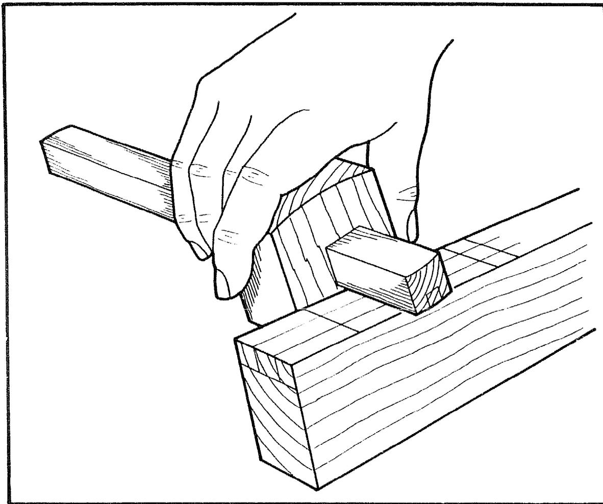
This design is based on the mortise gauges available in most tool shops. It is easy to use, but requires a higher degree of skill to construct.
