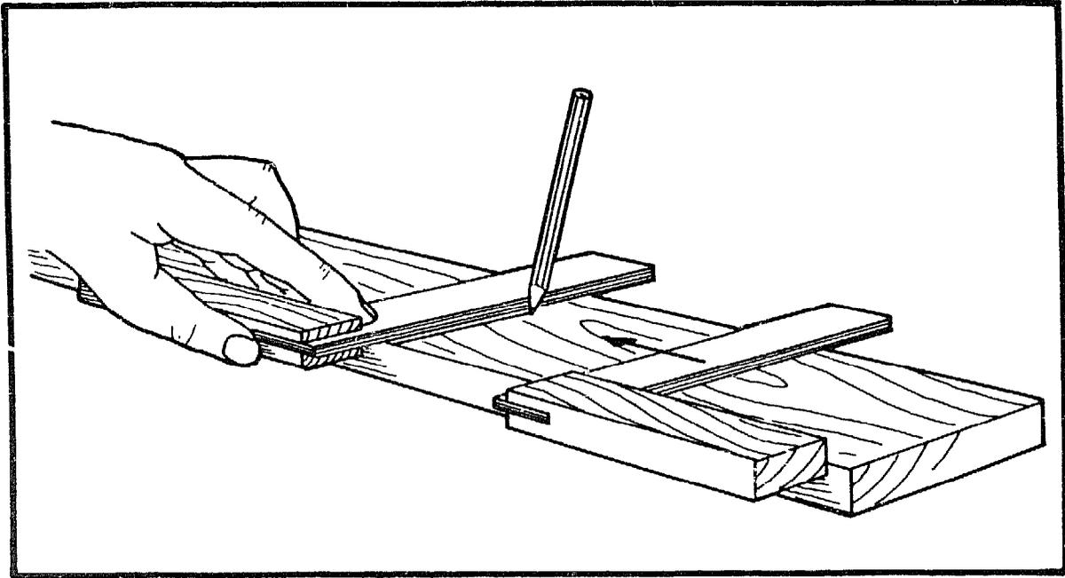
Take a piece of wood about 200mm wide, with face side and face edge planed straight and square. Place the try square on the timber and draw a line from the face edge. Turn the try square over to approach the line from the other side. If the square is true the pencil line and the straight edge will be parallel to each other.
