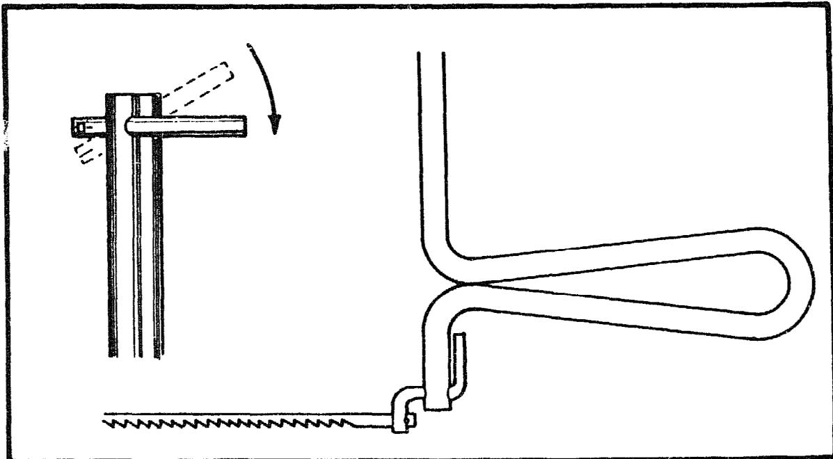
When using the coping saw make sure the blade is not twisted and the teeth point towards the handle. The blades are not strong so use the saw carefully.
