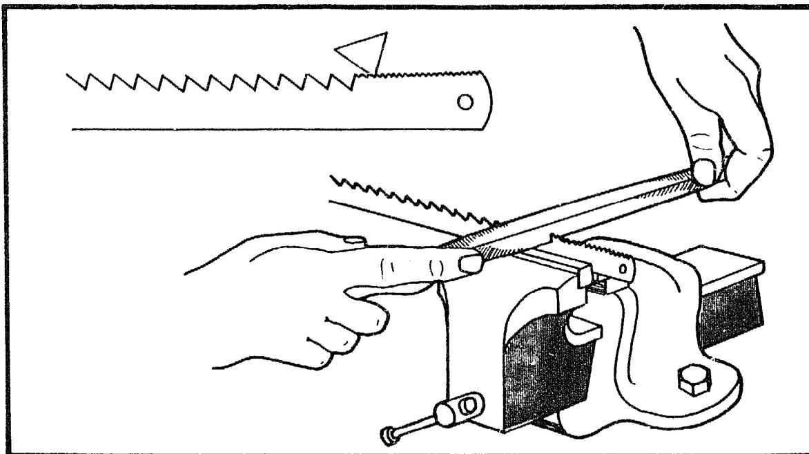
To make a blade for the Bow Saw, a hacksaw blade must be softened. Only the cheaper "low-speed" blades can be used. Put the blade into a fire until it is red hot. Take it out and let it cool down slowly beside the fire. With a saw file, file every third tooth until it is three times bigger. Take care to make each tooth the same size.
