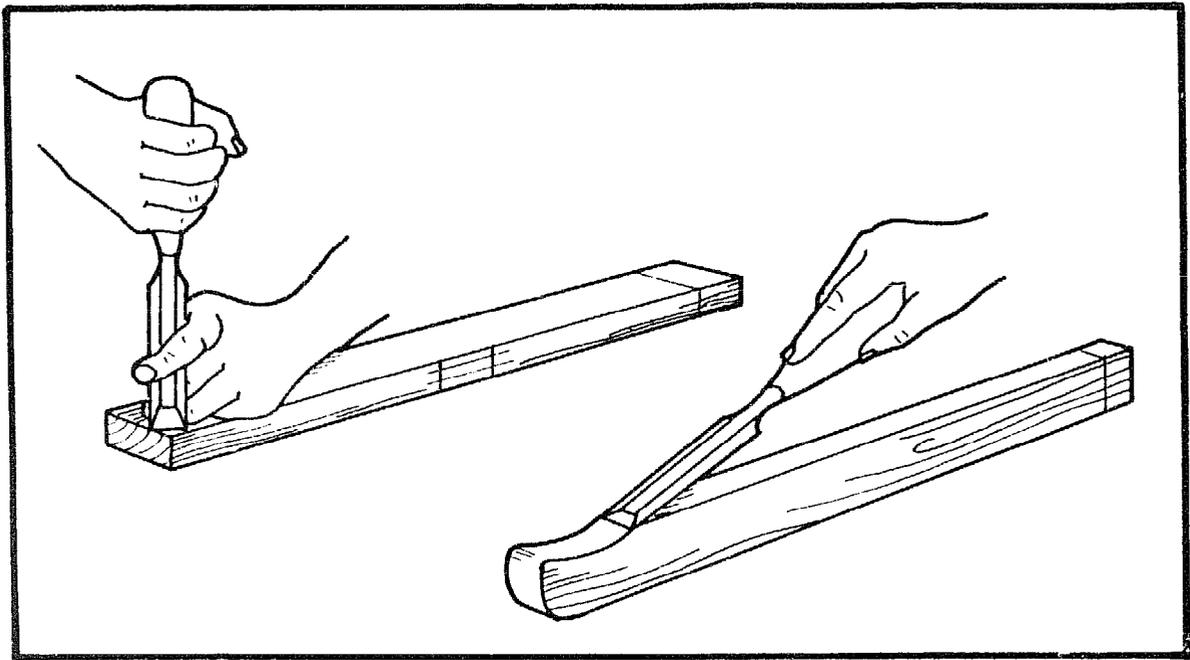
With a large chisel, shape the top of the side frames so that the string does not slip down. You can also round off the top inside corners.
