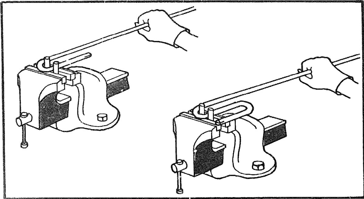
Make a 'U' shaped bending bar as shown on page 91. Heat the rod up and make the first bend 100mm from the end with the slit in. Heat the rod and make a second 180 degree bend opposite the end of the bar.
