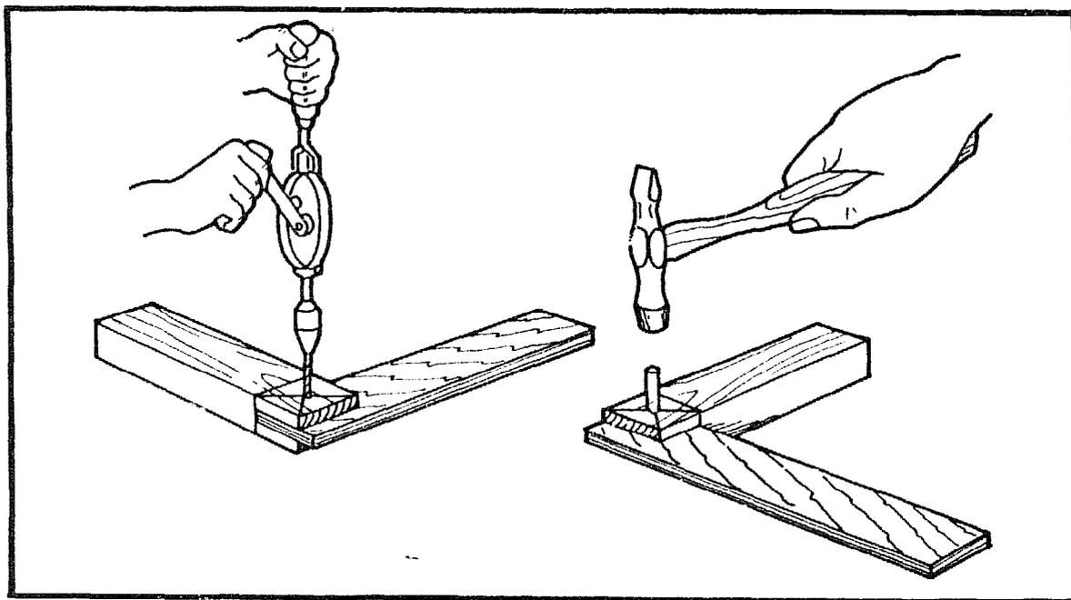
When the glue is dry drill a  $\text{Ø}6\text{mm}$  hole in the centre of the joint. Drive in a 6mm dowel. Plane the back of the blade flush with the stock and smooth up the ends of the dowel.
