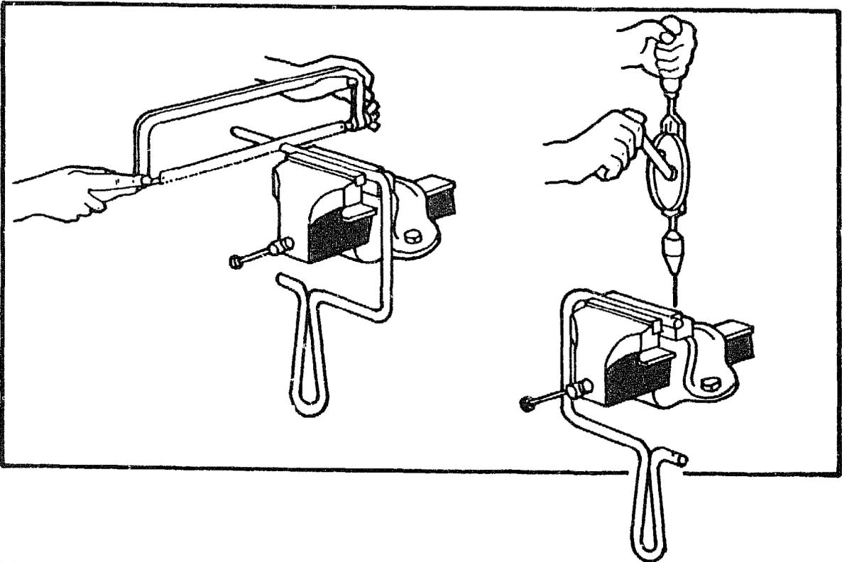
Measure and cut the front leg of the frame to be the same length as the leg at the handle. Punch and drill a hole the same size as the first, 10mm in from the end of the frame.
