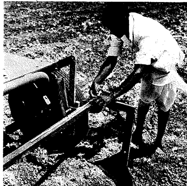
Check the distance of each ridger from the center of the toolbar and adjust if necessary to make it 75 cm.
