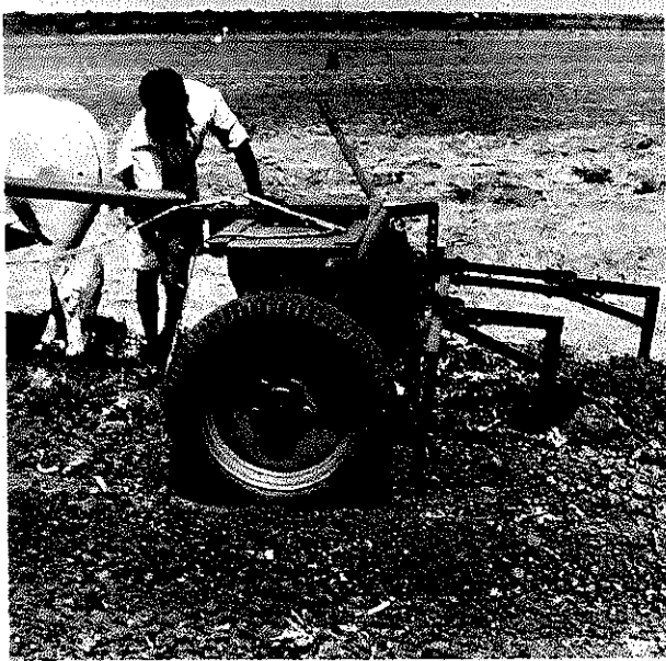
Adjust the pitch screw if the plow standards are not vertical.
