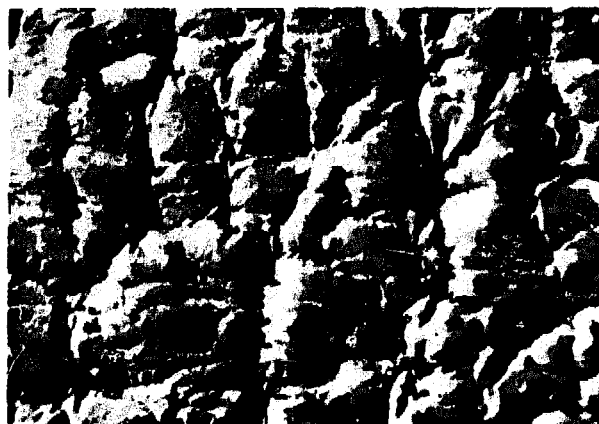
FIGURE 10. - Photo showing grain structure of dogskin (x 20).
