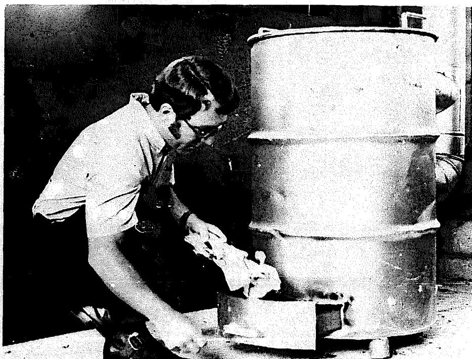
*Lighted paper is inserted into the drawer to ignite the sawdust stove.*
