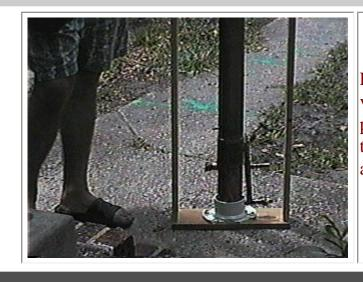
Lower section of completed still, showing the hot vapour inlet on the left, and on the right, the drain plug (bottom), the condensed run-off water outlet in the middle, and just above, the safety vent open to atmospere (45 degree angle fitting.)
