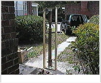
This is an alcohol fuel still, not a whisky still. It is designed for making 20 litres/hour of fuel grade alcohol. While it could be used to make whisky, it is larger and more expensive (it costs about \$500 to build). It takes a couple weekends to make it properly. People interested in energy selfsufficiency will find making alcohol a fun and a worthwhile thing to learn. You can turn thrown-away food into fuel.
