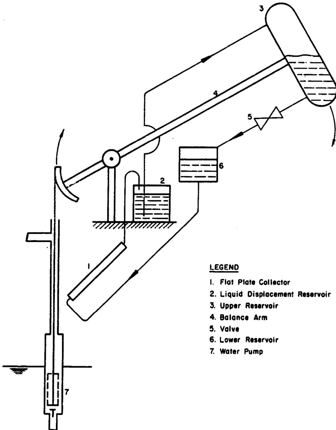
**FIGURE 47 - "CAMEL" GRAVITY OPERATED SYSTEM**
