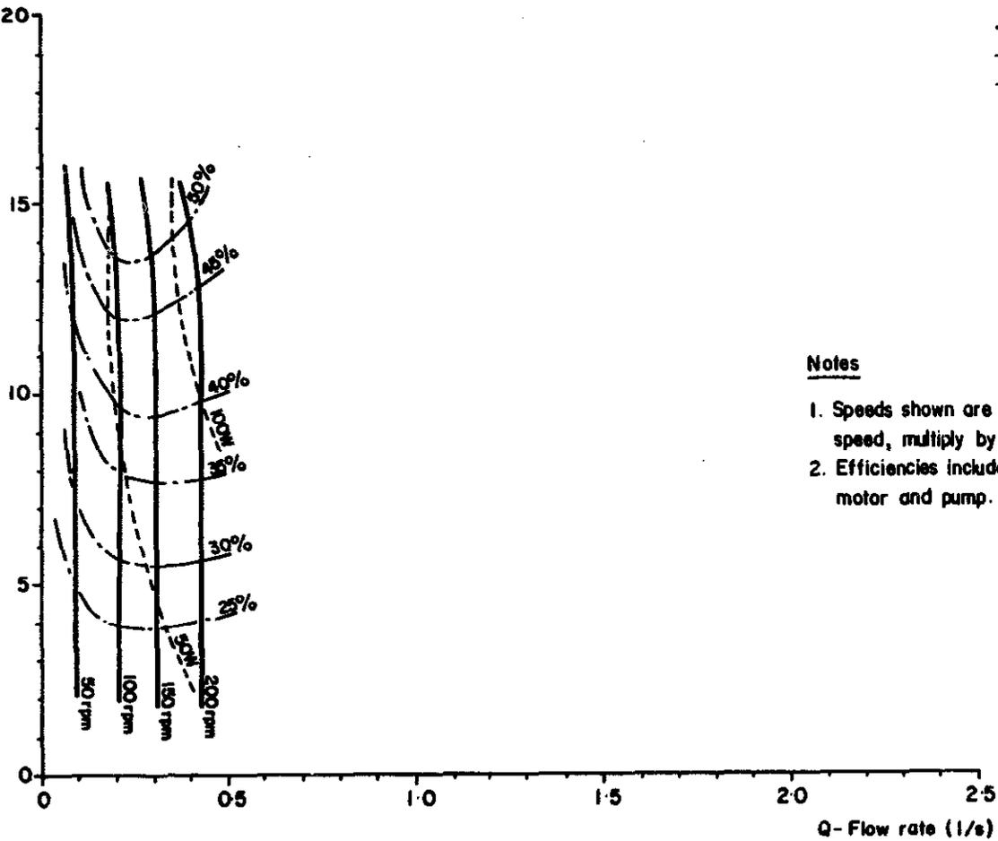
— Speed contours in rpm.
