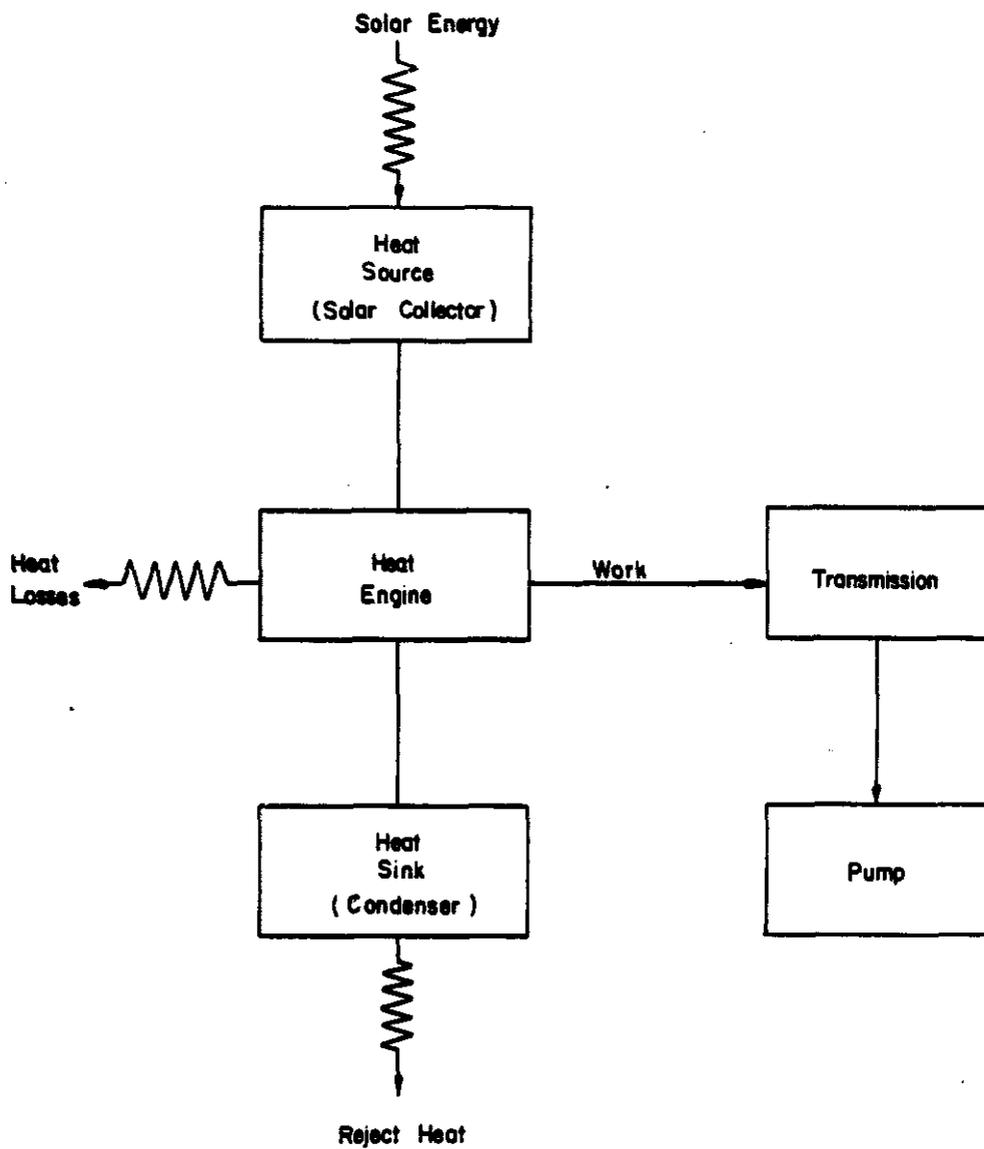
**FIGURE 42 – SCHEMATIC ARRANGEMENT OF A THERMAL SYSTEM**
