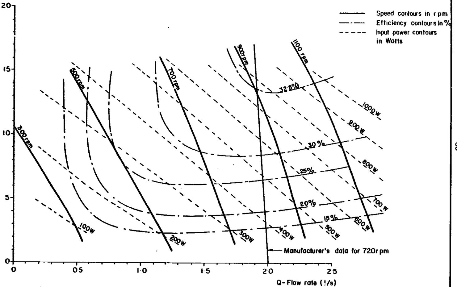
FIGURE 28 - TYPICAL ROTARY POSITIVE DISPLACEMENT PUMP PERFORMANCE
