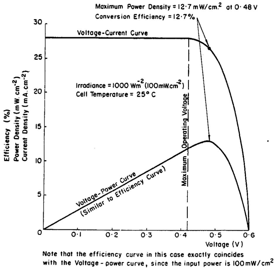
FIGURE 15 - VOLTAGE-CURRENT AND VOLTAGE-POWER CHARACTERISTICS OF A SILICON SOLAR CELL
