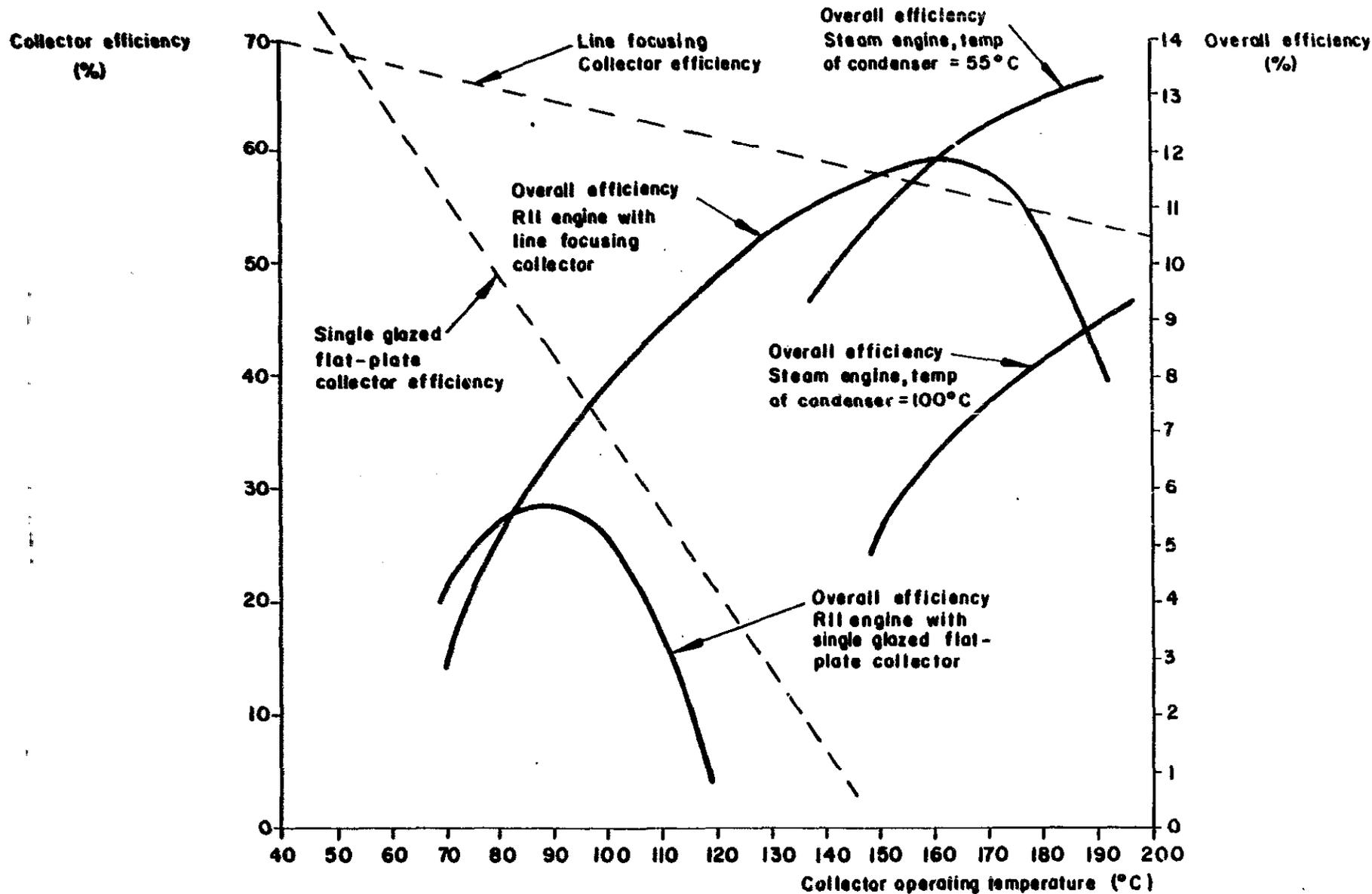
**FIGURE 51 - EXAMPLES OF SOLAR COLLECTOR AND ENGINE EFFICIENCY**
