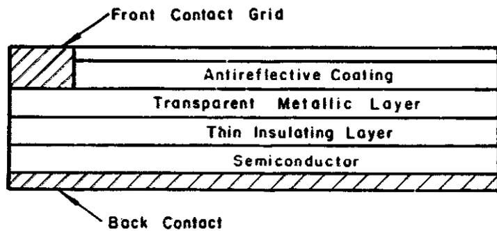
FIGURE 20 - SHOTTIKY BARRIER (MIS) SOLAR CELL
