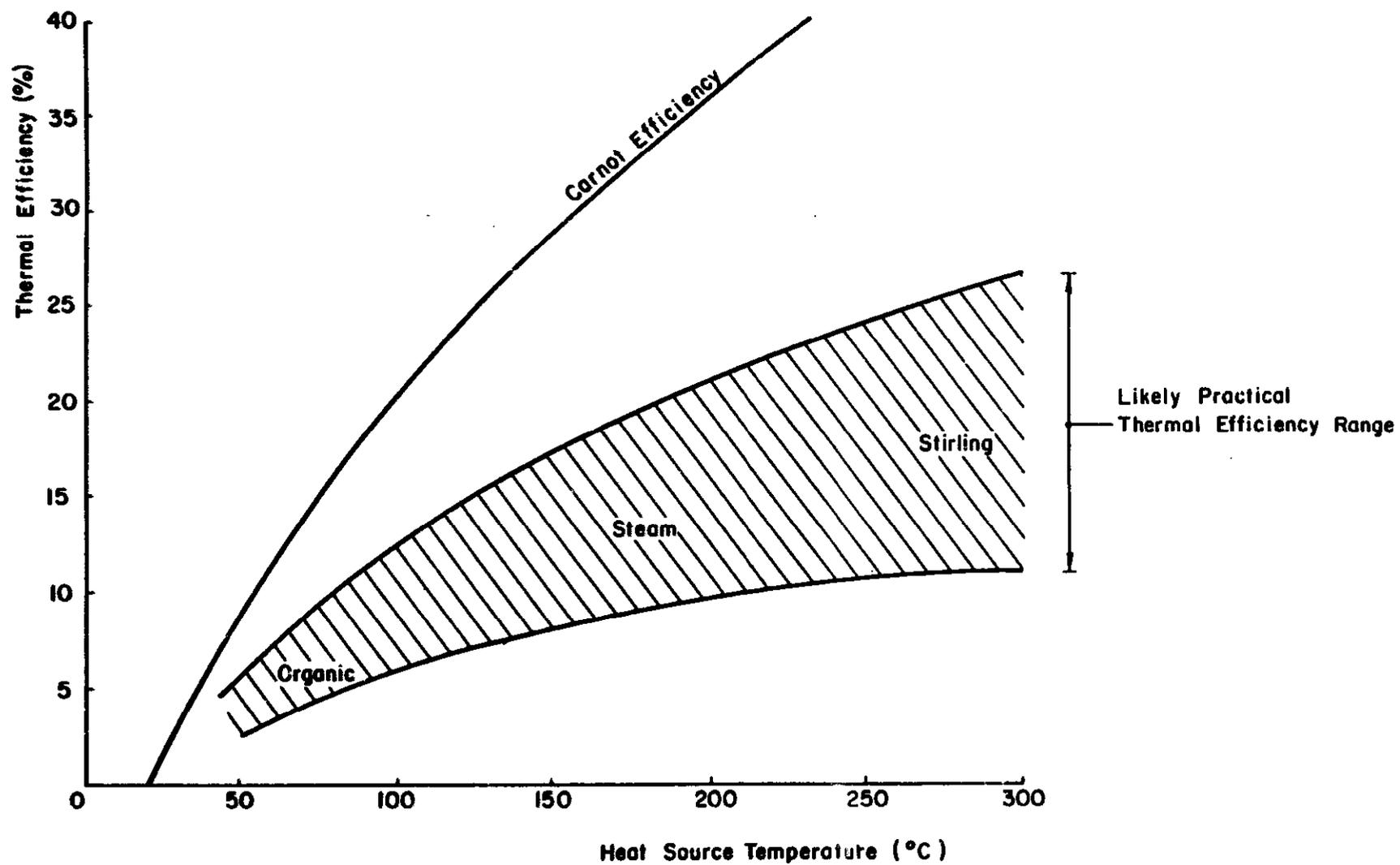
FIGURE 41 – COMPARISON OF THEORETICAL CARNOT EFFICIENCY WITH EFFICIENCIES OBTAINED IN PRACTICE ( $T_C = 25^\circ\text{C}$ )
