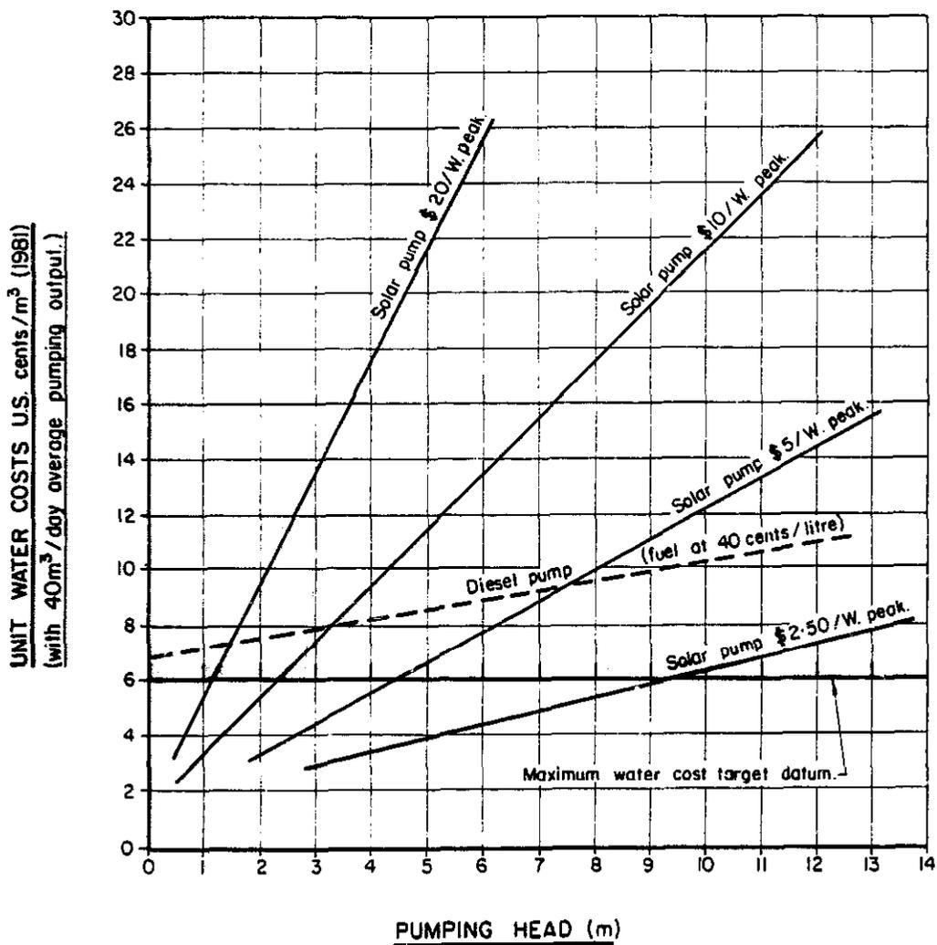
FIGURE 10 - EFFECT OF PUMPING HEAD OF WATER UNIT COSTS
