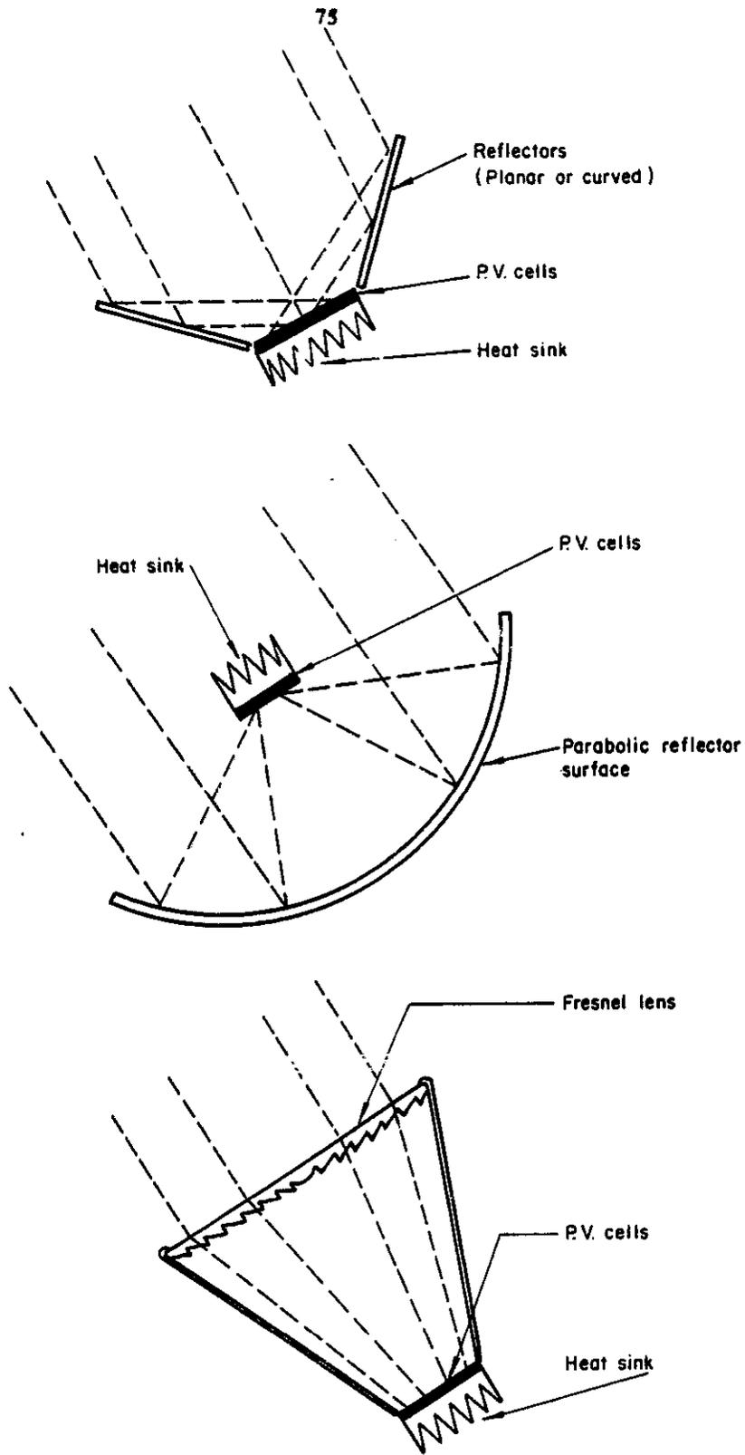
FIGURE 22 – METHODS OF CONCENTRATING SUNLIGHT ON PHOTOVOLTAIC CELLS
