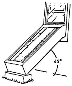
The plans attached show the complete assembly in addition to three sub-assemblies, cutting diagram and material list. It is suggested that the outer box be assembled, then the ' inner box, then the rear top sub-section. Then the sub-assemblies are combined. The sub-assemblies should be <u>caulked</u> using latex caulk on the inner corners and cracks. The outer box is caulked on the outside along cracks before painting. Place cover (Part 0) wi Insulation (CC) and insulation cover (W) on las
