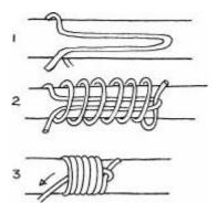
Very badly frayed or damaged ropes should be discarded. Ropes with one or more points of damage can be cut and the sound lengths kept for general purposes. Singe the ends of man-made fibre ropes to seal them. Use fine string (whipping twine) to whip the ends of natural-fibre ropes, as shown above.
