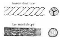
Hawser-laid polypropylene ropes are the type most commonly used for conservation work. Although these do not rot in water, they should still be stored dry and away from chemicals and batteries. Polypropylene ropes float, which is an advantage for pond work. Hawser-laid sisal or manila ropes will rot if kept damp.
