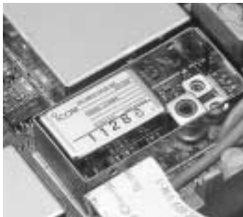
High-stability reference crystal oscillation unit
