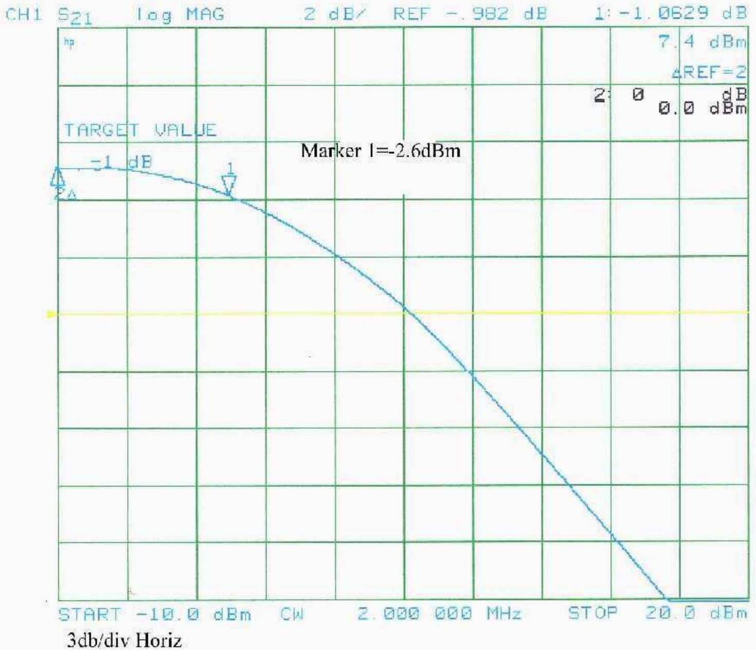
1dB compression is corrected to 8.1dBm output power.
