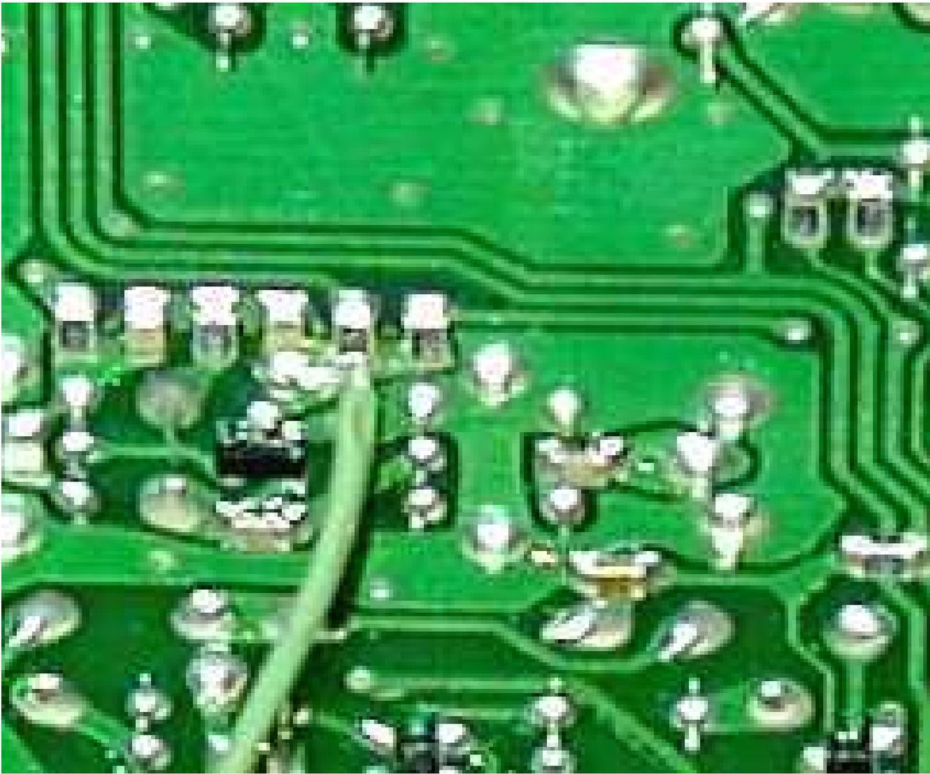
You can see the little black FET (Q1034) and the slightly triangle-shaped foil trace that connects to Q1034. I bent an "L" in the small wire I used. The wire will route topside to a terminal strip, so it needs to be several inches long.
