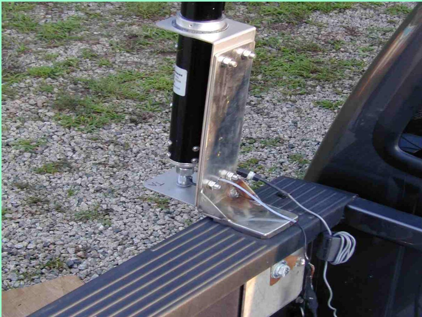
You can see where I get my shield ground connection. I feed the antenna with the single wire to the lug normally used to mount the impedance correction coil. I mount my impedance correction coils on PL-259 plugs so I can change them easily. I screw them into the SO-239 connector normally used as a feed!
