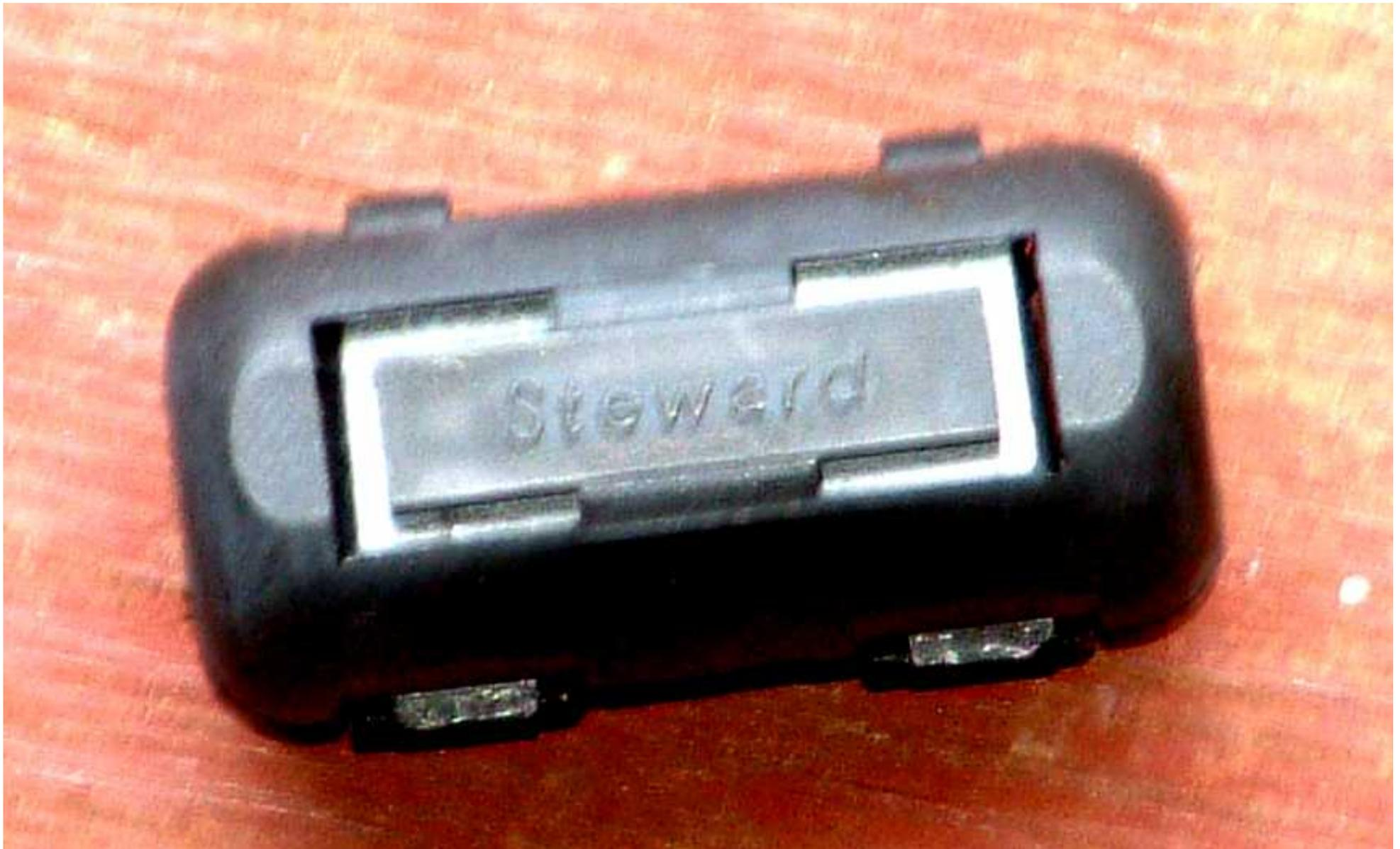
It is just over 1" long and about 1/2 inch diameter and snaps easily over RG58 or RG59 cables.
