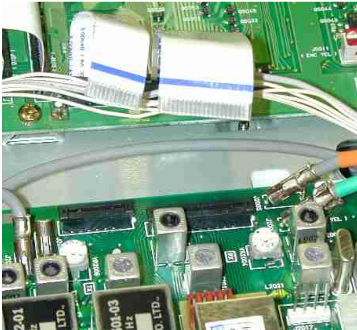
10.) Remove the mounting screws and flip the IF board exposing the bottom:
