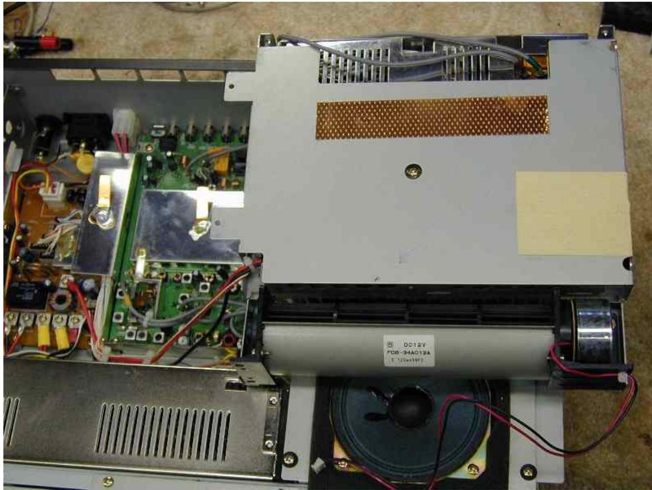
4.) The RF board is the green-colored board you see above. There are several screws holding that board down, and two screws on a rear panel DIN connector that is mounted on that board. The board will freely move when you remove ALL the screws. Do NOT pry or force the board out, if you have to pry you missed a screw!
