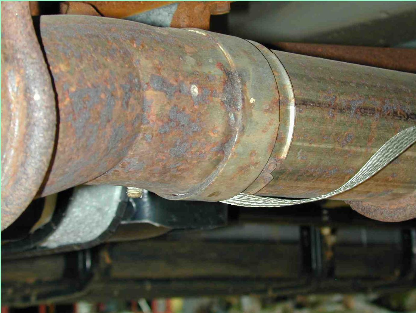
You can see the widening of the pipe as it expands into the muffler, with the fuel tank and transfer case in the background. The strap grounds under a nut used for the exhaust hanger. As before, I tin the leads and use stainless star washers to help maintain connections. Notice I clamped the strap under the factory exhaust joint clamp.
