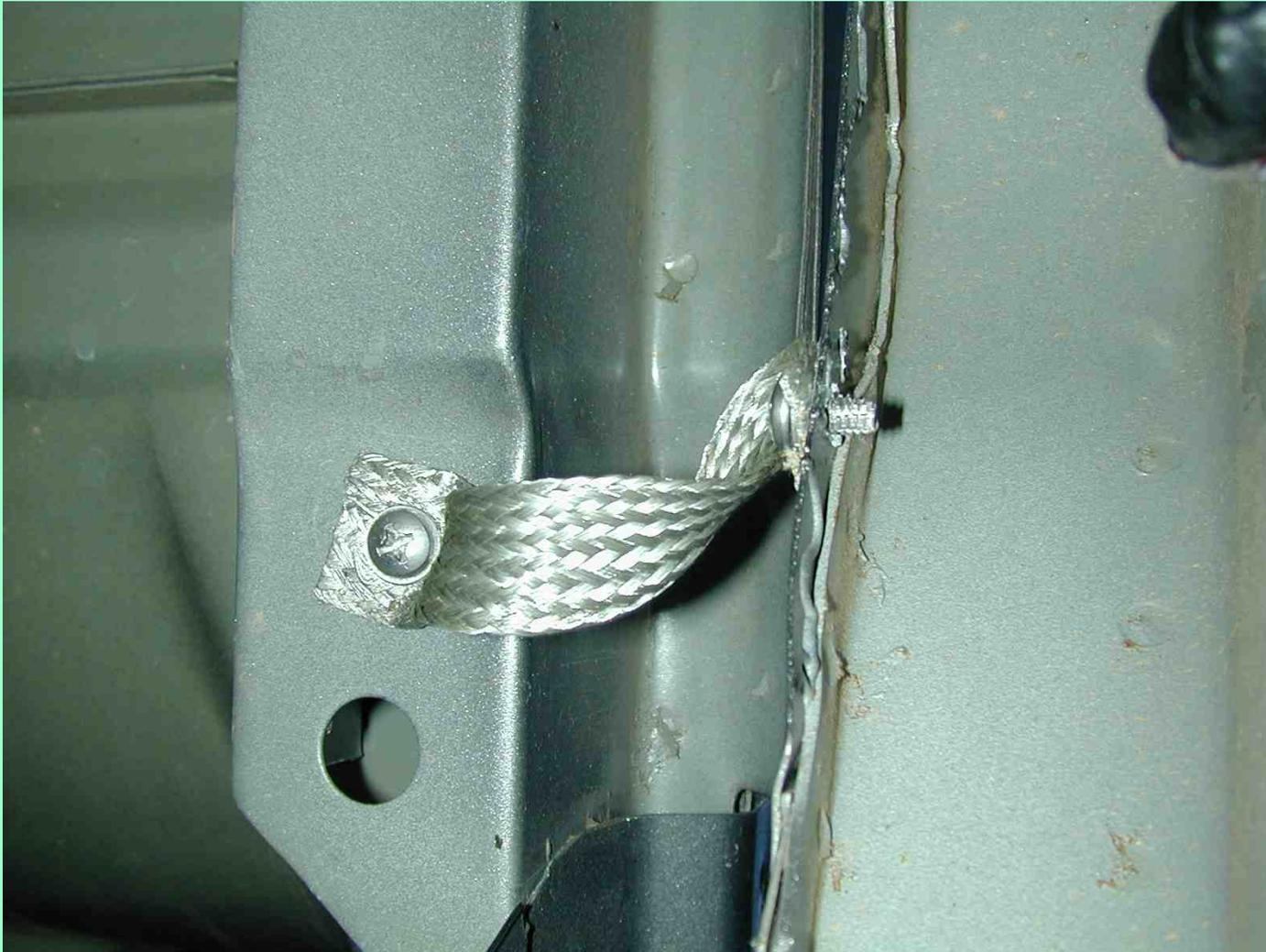
Note that I heavily tin the edges of the 1" braid. I do this insure all of the braided wires stay fully in contact all of the time. The flex area must remain solder free.
