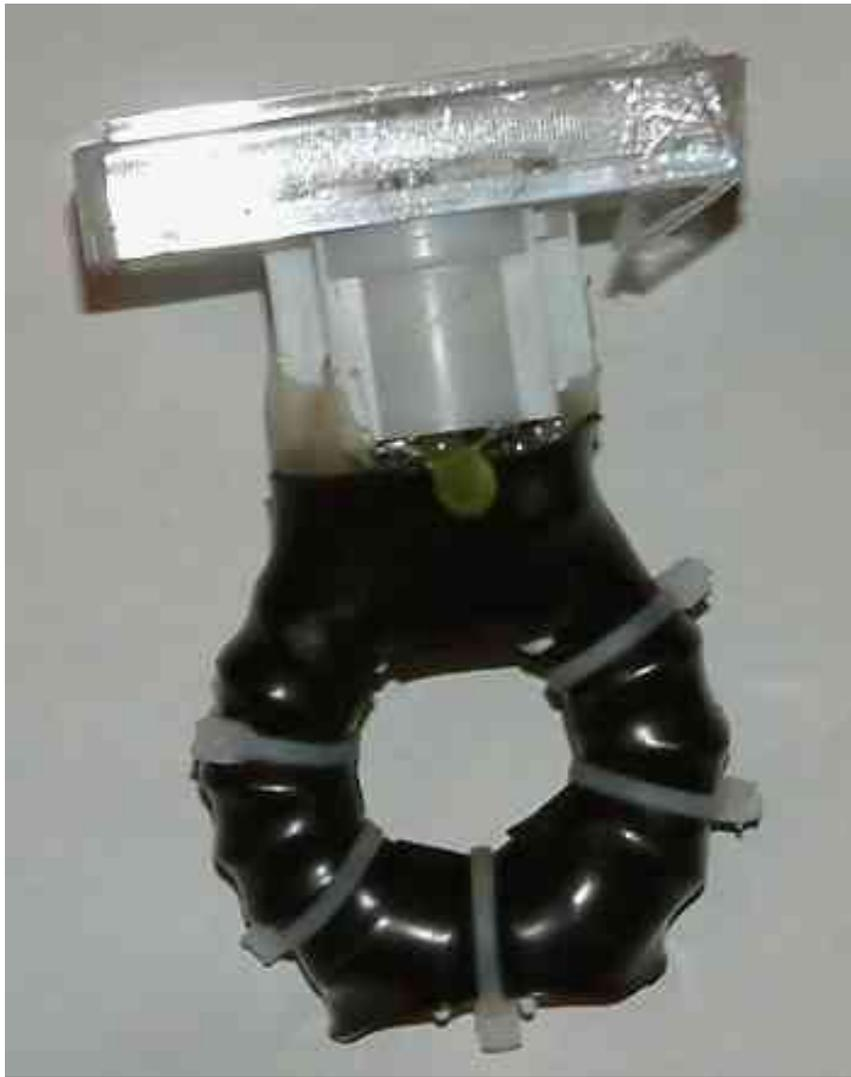
The meter has a low threshold Schottky diode detector, a series resistor for calibration, and standard .1uF bypass capacitors.
