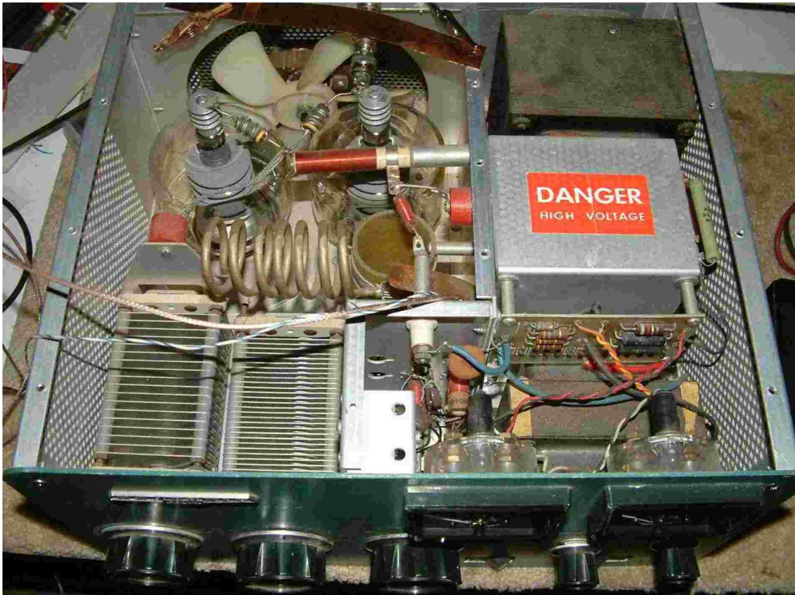
**The anode is excited with a swept power-leveled source feeding a bridging pad and the anode. The sweep is from 1 MHz to 300 MHz. The small coaxial cable and multicolored wire are from the high impedance J-FET source follower probe used to feed the second RF port of an Agilent network analyzer. In this condition the network analyzer acts like a sweep generator with a voltage detector.**
