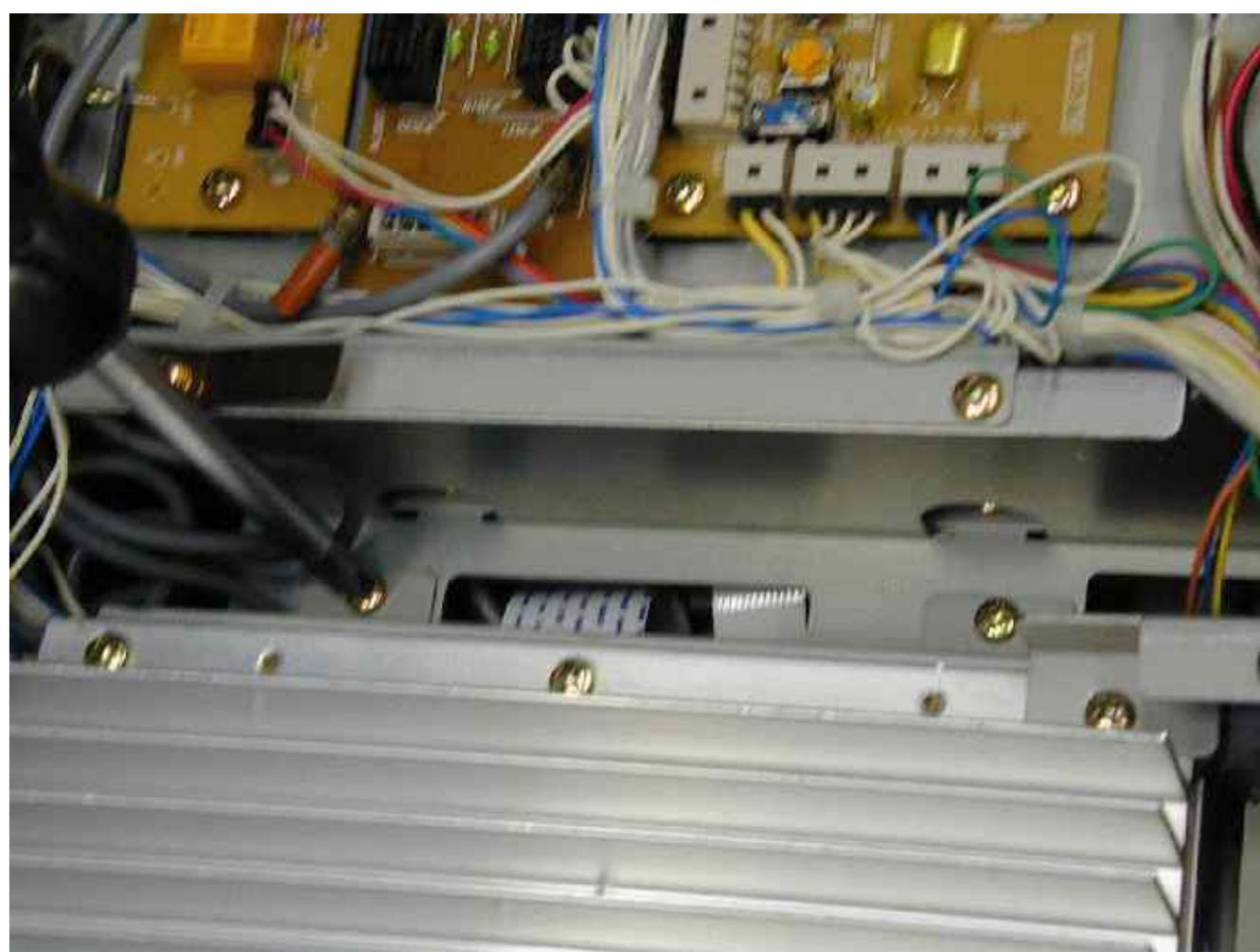
Four main screws hold the heatsink mounting bracket. Two are shown above (one under the screwdriver and one to the right of it). Two other screws are on the side of the radio chassis. You might want to remove the long screws holding the fan bracket, although I got by without doing so.
