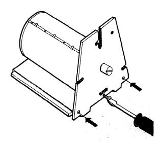
4 Join the second side panel to the base using three screws
