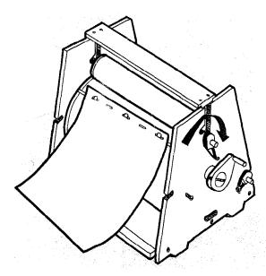
9 Put the pressure roller into the working position
