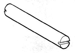
One disc should be glued centrally on the shaft and the other two discs should be glued approximately 2½" from the ends of the shaft such that their other surfaces are 10½" apart. This should leave approximately 2½" of shaft at each end
