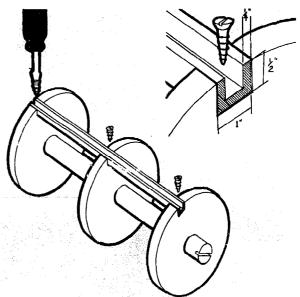
6 Use a piece of tin plate or 1mm plywood to cover the wooden discs. Join the tin plate to the wooden channel section with tacks. Leave a gap to put in the fabric grip
