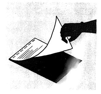
8 Hook the stencil with the backing paper attached on to the metal clips on the stencil drum
