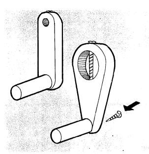
Join a length of dowel to the handle and attach it using a countersunk headed screw
