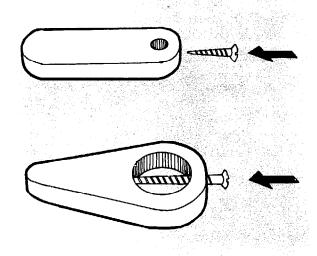
To attach the handles to the shafts put a screw of minimum length 1%" through the end of the handle
