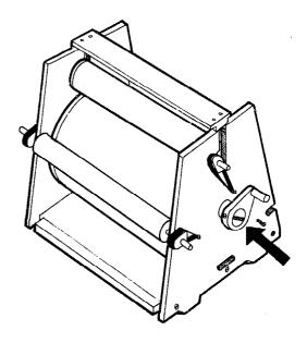
4 Put the ink along the roller in the trough between the roller and drum
