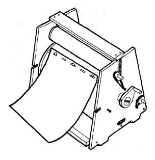
10 Remove the handle from the stencil drum and attach the pressure roller handle to the pressure roller
