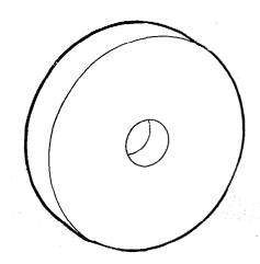
2 Cut from each disc a channel for putting in the fabric grip (item 3), %" deep and 1" wide, drill a 1" diameter hole in the middle to take the shaft
