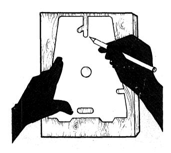
3 Cut out along the lines and sand all surfaces before assembling the duplicator
