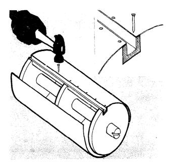
7 Cover the stencil drum with felt or absorbent material, allowing the material to overlap. Cut out the fabric grip from a strip of hardwood %6" square and 10½" long. Put the fabric grip into the channel on the stencil drum. This will tighten the fabric around the drum. Trim as required then secure the fabric grip to the stencil drum with screws
