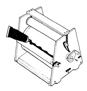
Turn the stencil drum handle back and forth to spread the ink over the roller. Make sure you only ink the area which will be covered by the stencil (you do not even need to ink the outer edges of the roller as you will not type to the very edge of the stencil). Do not use too much ink and do not cover the complete stencil drum or you will ruin the stencil and rollers
