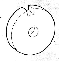
3 The shaft is made from 1" diameter dowel cut to a length of 15". To locate the handle cut a groove into each end of the shaft
