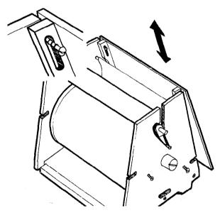
3 The top cover panel (item 13) should fit underneath the case handle (item 7)
