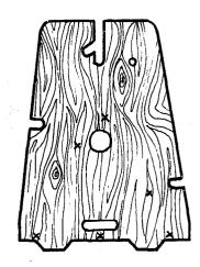
2 Using template 3 cut out the base from %" thick planed wood and make a groove %" deep for inserting the deflector plate (item 4)
