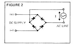
paths for current flow from the DC source to the AC lines, arranged so that each path is suitable for power flow to the line in one of the half cycles during the interval that corresponds to the D area in figure 1.
