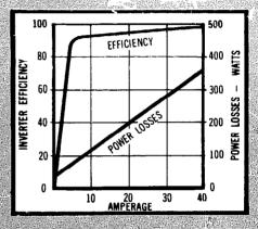
In addition to minimizing system losses associated with current level, operating at higher voltages results in a minimum VAR load imposed on the AC lines.
