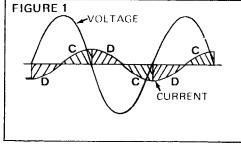
can be seen in figure 1, showing the AC voltage and current waveforms of a single phase line supplying an inductive load. Although a purely inductive load consumes no power, current flows through the load, and power is instantaneously traded back and forth with the AC lines.
