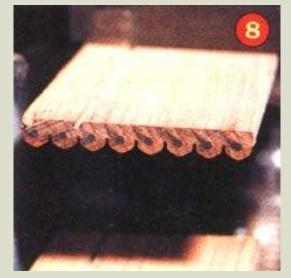
When the glue dries, the slats are fed through a cutting machine. Fast revolving steel blades trim the wood into round or hexagonal shapes, one side at a time.
