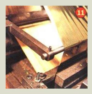
A heated metal stamp presses the name of the company and a number (such as the number 2) on the pencil in gold foil or in paint. The number indicates how hard the pencil lead is.
