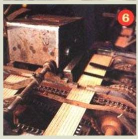
In another part of the factory, the wood is prepared. Machines cut blocks of cedar into wide slats. Eight shallow grooves are sawed lengthwise into each slat.
