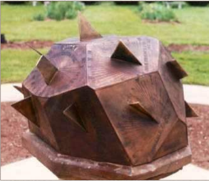
A polyhedral dial with faces oriented to tell time in various world cities.
