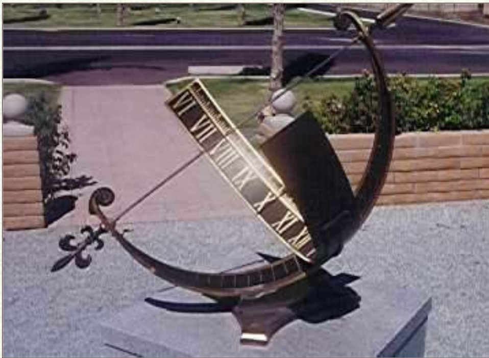
Another form of the equatorial dial, often called a "bowstring" equatorial
