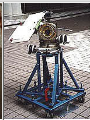
Photo P10- Sunlight-2 heliodon, testing a horizontal sundial
