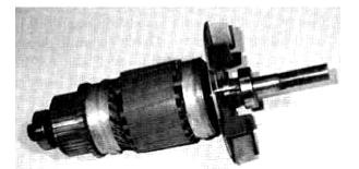
FIGURE 12-2 The armature (rotor) of a DC motor has coils of wire wrapped around its core. The ends of each coil are terminated at commutator segments located on the left end of the shaft. The brushes make contact on the commutator to provide current for the armature.
