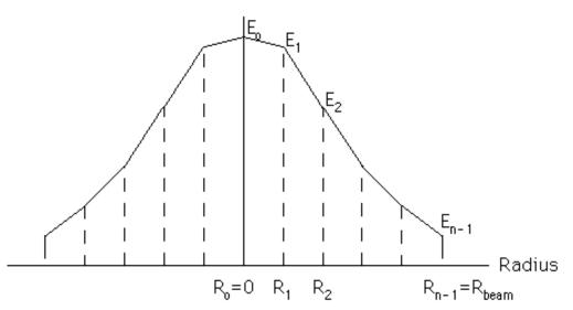
Beam radius is divided into n equal part (radiuses and illumination reading values are indexed from 0, at the beam center, to n-1, at the beam edge).
