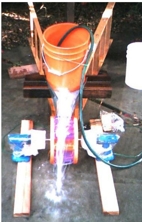
I also tested a 1/8" water hose nozzle blasting water out at city water pressure (about 45 lbs/Sq. Inch). This approach would charge two cells at about .45 amps and one cell at about .5 amp or .8 watt. This approach uses the inertia of the water. Both generators were wired in series. See <http://home1.gte.net/mikelob/WaterW-9.JPG> for the setup.
