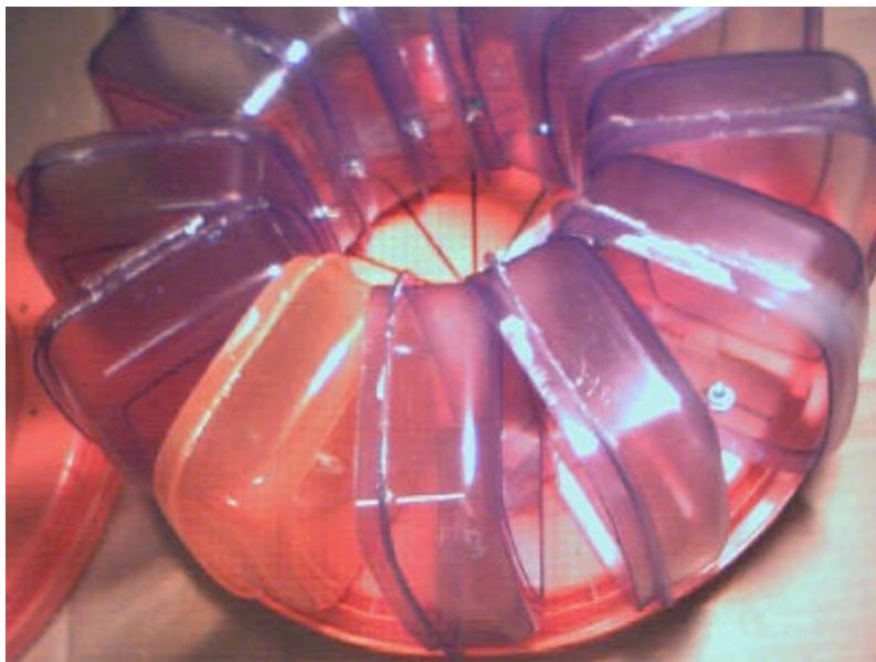
Mark and drill holes in one lid then use this lid as a guide to drill the holes in the other lid. Add a ring of “silicon-I” sealer and centered the now circular ring of plastic containers and drill-bolt the buckets to the lid.
