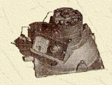
This hydroelectric battery charger uses a cast bronze pelton wheel and an 80 amp Ford alternator in a powder coated aluminum housing. We can supply the turbine with one, two or four nozzles, depending on water flow and power requirements. These turbines can be fitted with nozzles up to 1/2" in diameter.
