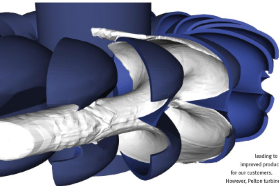
Fig. 2 (above): Predicted water jet deformation as it interacts with three buckets, showing thin water sheets leaving buckets.
