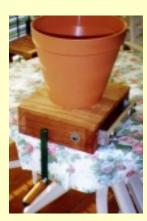
Its basically the same design as my none adjustable model, running on bearings and solid stainless steel rollers. The metal frame sticking out the side has one of the rollers bedded in it, and that is how you adjust the gap.
