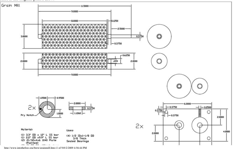
(2) 21/32x4x6 1040 Plate (Painted) (2) 2' 00 SS offset ring: 3/8 Thick Sealed Bearings
