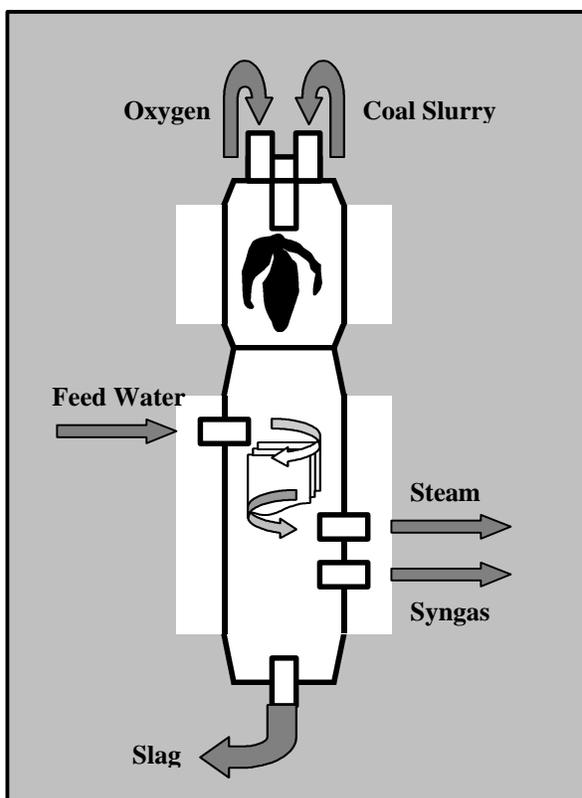
cooled to 450°C prior to going through a cyclone and a filter that retains most of the fly ash and the char particles. The collected fly ash and char is reinjected into the gasifier by a pneumatic transport system using nitrogen. The halides and sulfur compounds in the syngas are removed and the syngas is sufficiently cleaned to comply with the tolerance limits of fuel cells and gas turbines.
