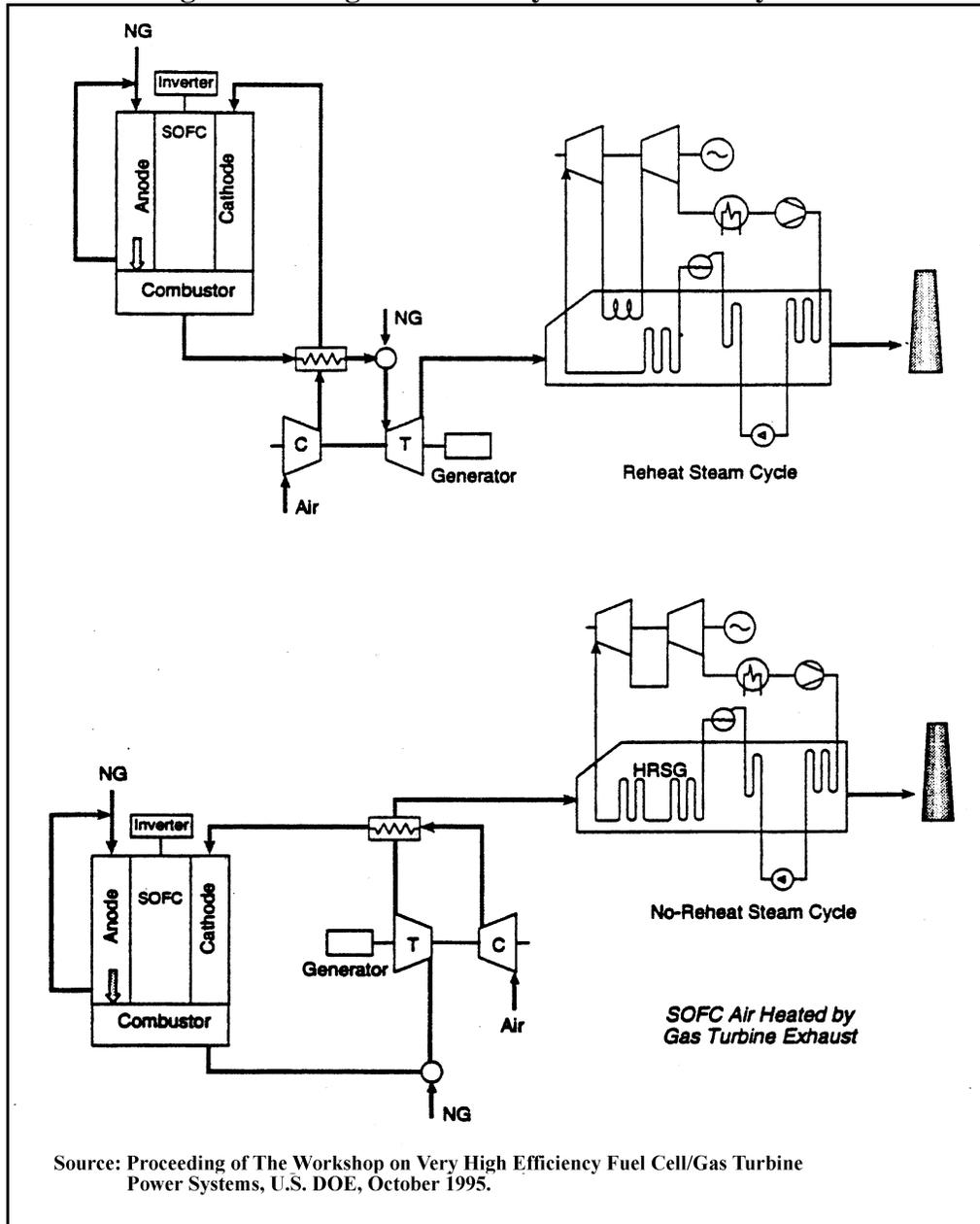
Figure 5.5 - Advanced Fuel Cell Hybrid System
