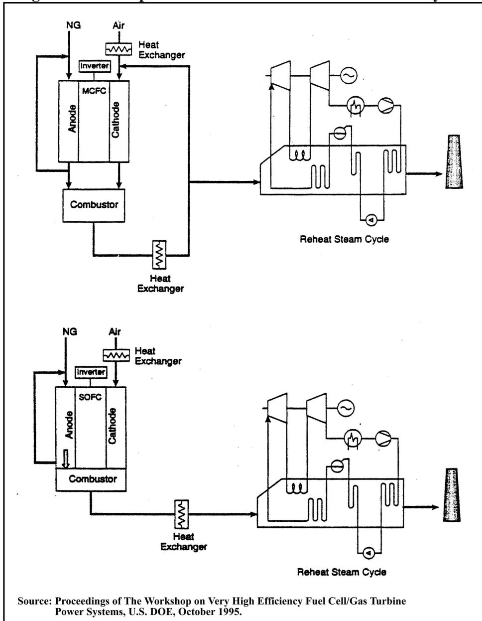
Figure 5.3 - Low Pressure Hybrid Fuel Cell System
