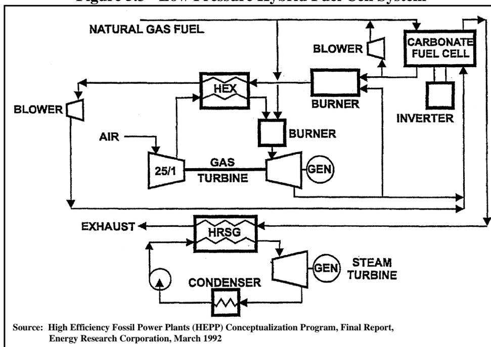
In a pressurized system (Figure 5.4), air is first pressurized for use in the fuel cell and waste fuel from the fuel cell anode and cathode exhaust, is then combusted to drive a turbine generator. The turbine exhaust is then used to generate steam to drive a steam turbine.
