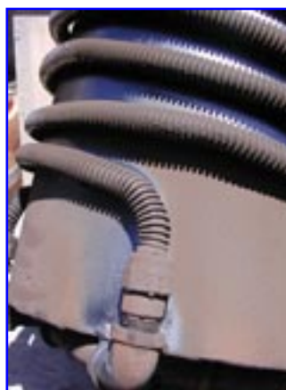
GEK Report #1: Air Preheating Tubes: Zero Tar Gas
