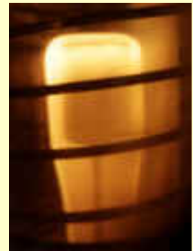
One inch birch dowell pyrolysing at 600C
