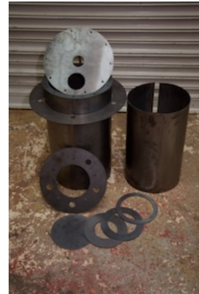
Downdraft Reactor Tubes, Flanges, End Plates, and Reduction Bell Weld Rings
