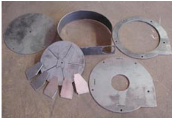
Rotary ash grate, gas cowling and swirl burner
