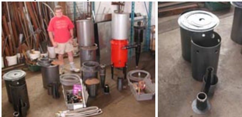
GEK kit at various levels of part count, welded state, and assembly/disassembly
