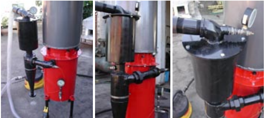
Newly combined cyclone and packed bed filter
