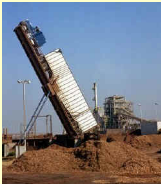
Truck unloading wood chips
