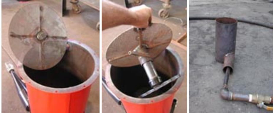
Rotary ash grate, gas cowling and swirl burner
