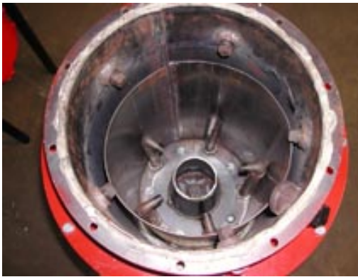
Air preheating / syngas cooling stainless steel heat exchanger
