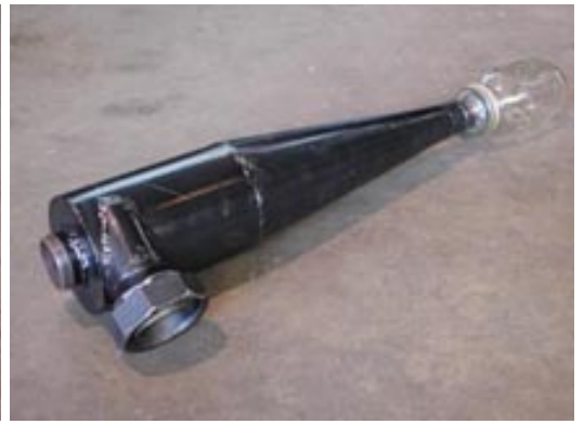
Air preheating / syngas cooling stainless steel heat exchanger
