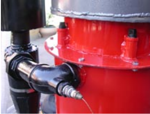
Newly combined cyclone and packed bed filter
