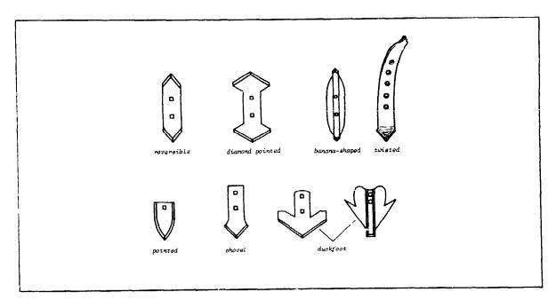
Fig. 41. Chisel shapes.
