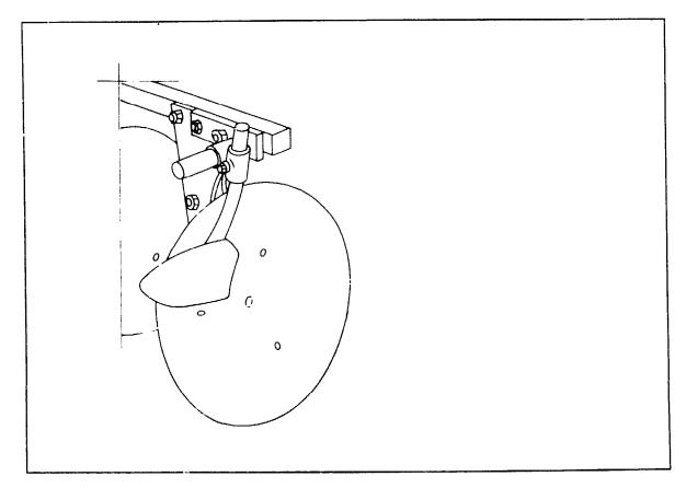
Fig. 31. Disc with scraper.
