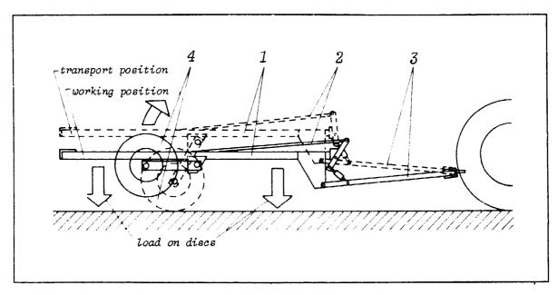
Fig. 53. Hitching device to enable both a full load transfer of the implement mass on to the discs as well as a correct levelling. 1. Frame.
