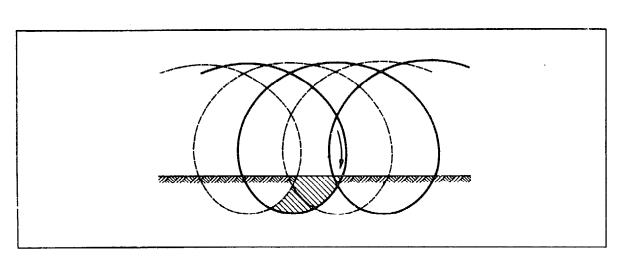
Fig. 44. Cycloidal paths of points on the cutting edge of two consecutive knives of one working set of a rotary tiller.
