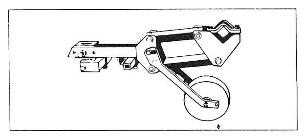
Fig. 104. Paralellogram mounting for ridgers.
