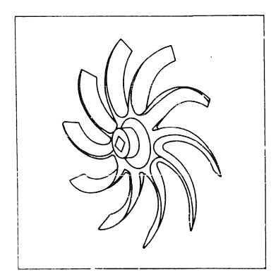
Fig. 64. Spider wheel (cast iron):
