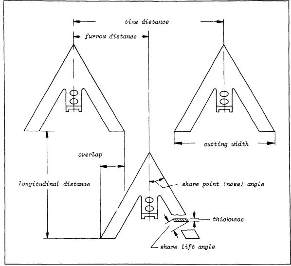
Fig. 121. Tools.of a sweep plough.
