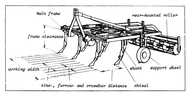
Fig. 38. Parts of a chisel plough.
