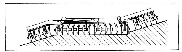
Fig. 56. Disc harrow with articulated frame for undulating surfaces.
