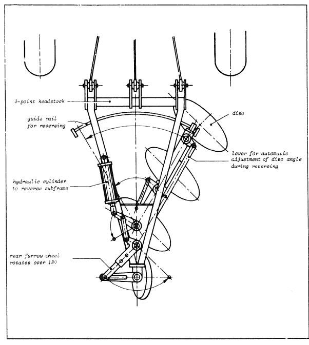
Fig. 30. Three-furrow reversible disc plough.
