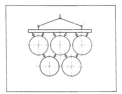
Fig. 90. Hoop-leveller (drag type).
