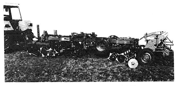
Fig. 144. Multitiller with leveller and rear-mounted drill.
