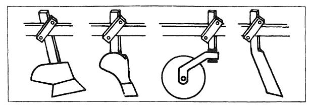
Fig. 24. Front-mounted tools. From left to right: jointer, manure feeder, disc coulter, knife coulter.
