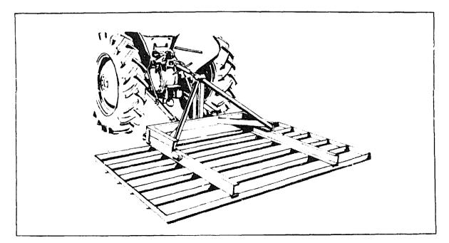
Fig. 88. Leveller (3-point hitch type).
