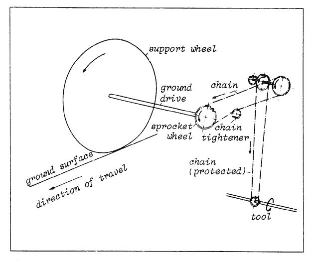
Fig. 125. Drive system of a rod weeder.
