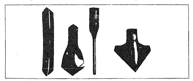
Fig. 72. Chisels for light cultivators: From left to right: standard (pointed) chisel, duckfoot chisel for stubble, grassland chisel for pasture, duckfoot chisel for tillage in row crops.
