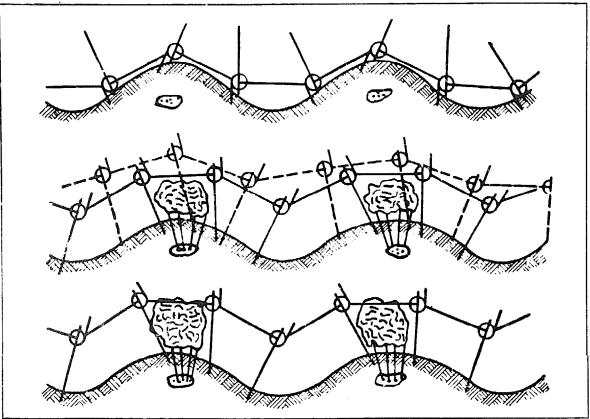
Fig. 97. Spiked-chain harrow operating on ridges.
