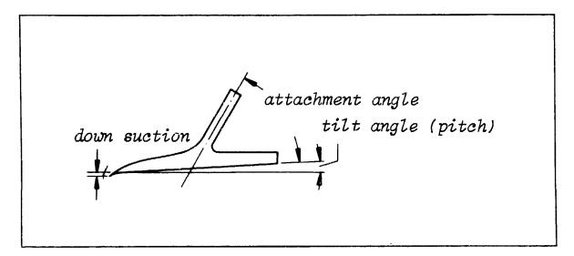
Fig. 123. Geometry of a sweep.
