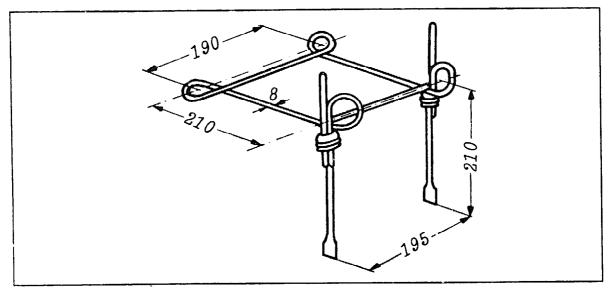
Fig. 98. Link with times of a spiked-chain harrow.
