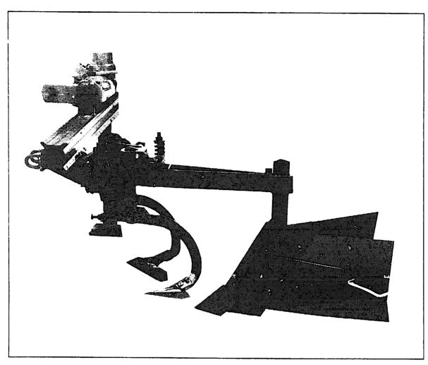
Fig. 112. Ridging body with duckfoot chisels running ahead.
