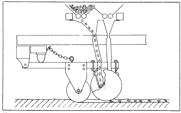
Fig. 132. Direct drilling unit (side view).
