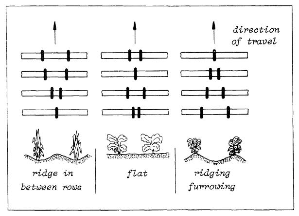
Fig. 70. Arrangement of the tines of a light cultivator with four crosswars in ridge and bed systems.
