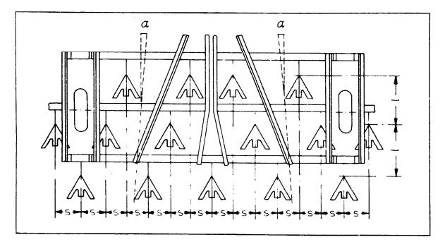
Fig. 120. Sweep plough with symmetrical arrangement of tools.
