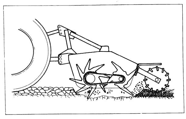
Fig. 78. Dual-rotor combination.
