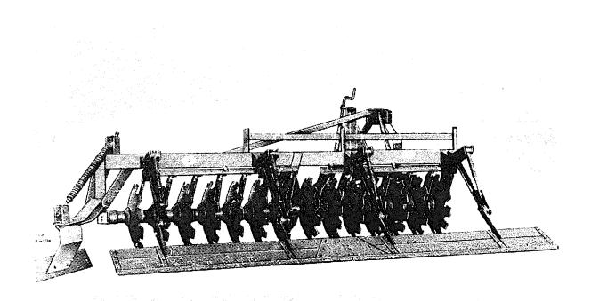
Fig. 118. One way tiller (3-point hitch, cut-out discs).
