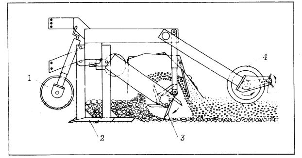
Fig. 137. The main parts of the "Justus": 1. Disc roller, 2. Sweeps, 3. Tine rotor, 4. Packing roller.
