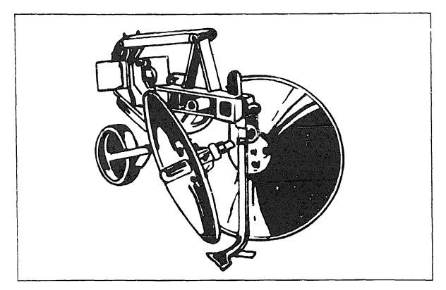
Fig. 110. Disc ridger with two discs.
