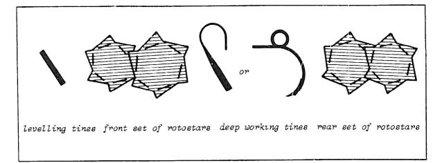
Fig. 143. Tools of the Multitiller (side view with two alternatives for the deep working time section).
