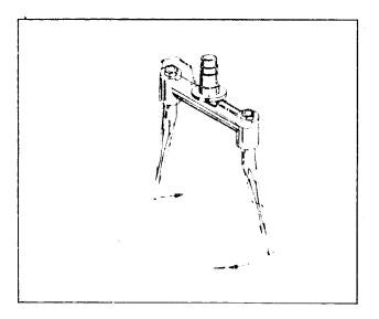
Fig. 84. Tool carrier with two tines.
