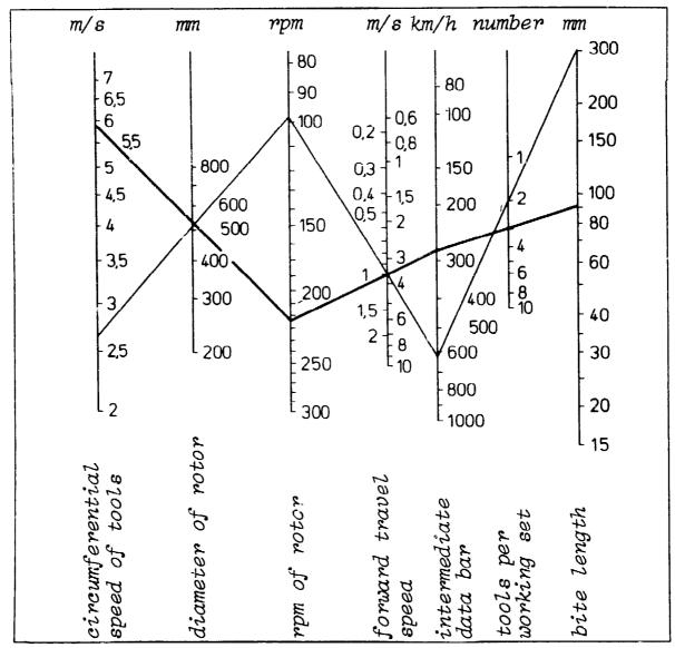
Fig. 51. Bite length as a function of design and adjustment for a rotary tiller. Based on the required bite length (extreme right aris), the possible combinations for adjustment can be found.
