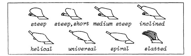
Fig. 23. Various mouldboard shapes.
