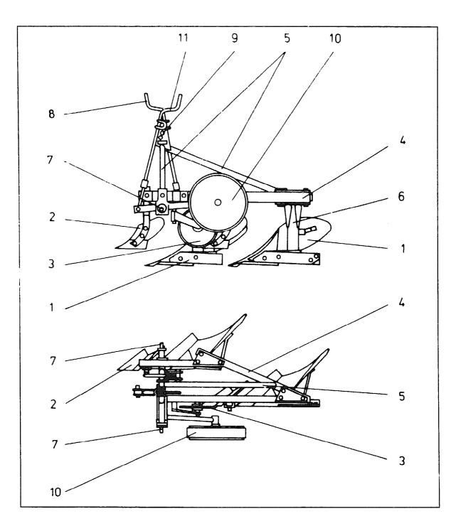
Fig. 18. Mouldboard plough (two-way, mounted) after Bernacki. 1. Body,
