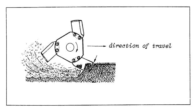
Fig. 45. Clearance angle of rotary tiller knives (indicated by arrow).
