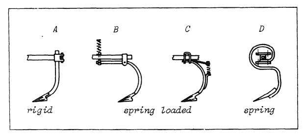
Fig. 39. Chisel tine shapes.
