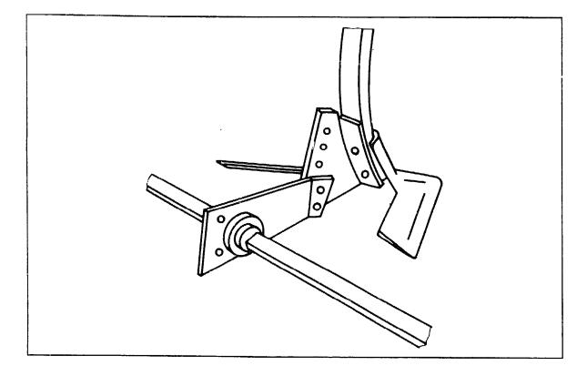
Fig. 124. Rod weeder mounted on a sweep plougn.
