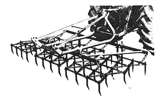
Fig. 67. Harrow with three sections in suspending frame.
