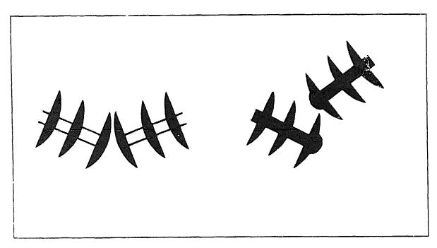
Fig. 57. Arrangement of the front disc gange. Lej't: overlapping action of center discs, right: center strip left untilled.
