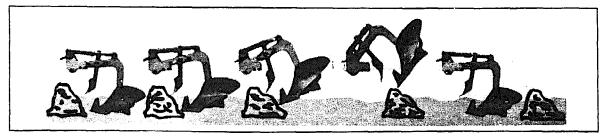
Fig. 26. Safety devices (protection against rocks and stumps) on a mouldboard plough.
