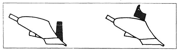
Fig. 25. Body-mounted tools. left: coulter, right: trash board.
