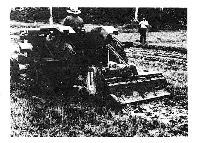
The small two-wheeled or walking tractors are an important group of implements used primarily for tillage operations. These implements are included in this chapter because they are developed and used extensively in paddy production systems in the Far East and especially in Japan. In 1979 330,000 of these "power tiller" units were manufactured in Japan, approximately 100,000 of them for export.
