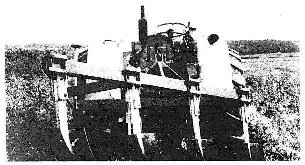
Fig. 147. Spade plough (rear view).
