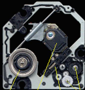
Spindle Platter Pickup Rack Gears Sled Drive
