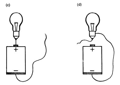
Most articles and systems using electricity have a switch which works by disconnecting one of the wires, so the electricity cannot pass through.
