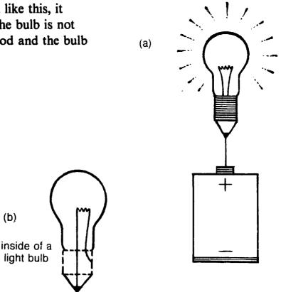
If either wire is loose, the electricity will stay in the battery, and the bulb will not light.
