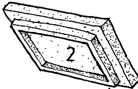
When box has been assembled and glued, cover interior surfaces with kitchen foil.
