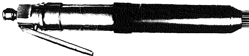
Figure 8. Needle impact scaler.
