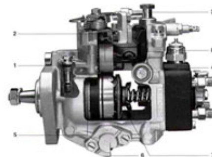
Cutaway view of an injector pump -- complex, expensive
